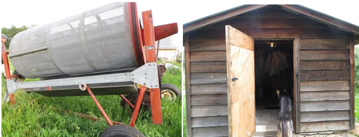
Figure 19. Seed Cleaner pictured left. Root cellar pictured right. The root cellar shed is built on top of a six foot diameter vertical culvert dug into the earth. This cellar stores thousands of pounds of root veggies up to 8 months in perfect condition.
