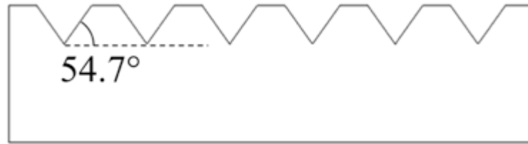
Figure 3.6: Cross-section of the V-groove grating.
