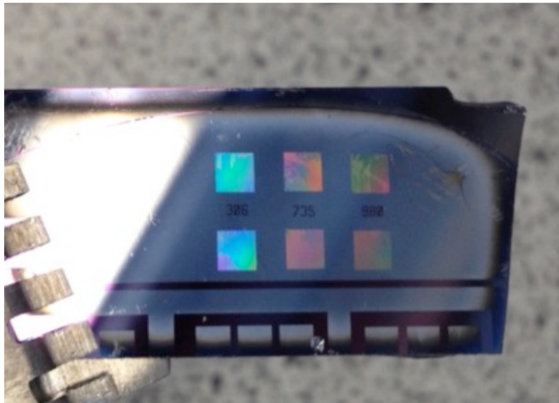
Figure 3.1: Picture of fabricated blazed grating.
