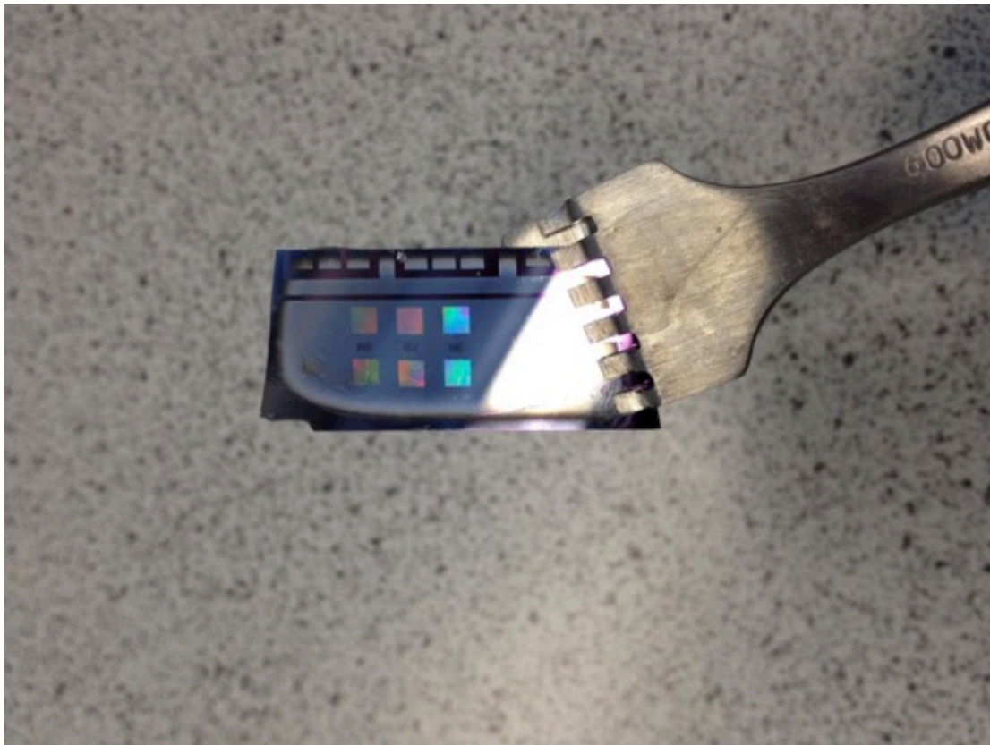
Figure 3.14: Grating sample after oxidation sharpening.
