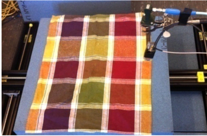
Figure 4.10: The picture of the experiment setup. The gun-shaped target is placed on the x-y stage and covered by a piece of cloth.
