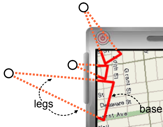
Figure 15: The Wedge off-screen pointing technique. The pair of legs point toward the target, converging off-screen at the position of the target. The base connects the legs and completes the shape.
