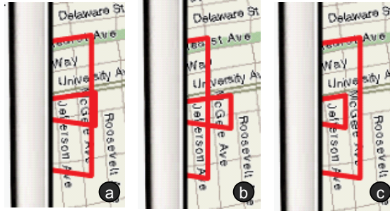
Figure 19: Two overlapping wedges shown in each of the three options for leg length: a) constant leg intrusion; b) shorter leg intrusion for further targets; c) longer leg intrusion for further targets.
