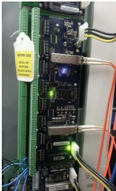
Figure 3-9: RTDS digital input card (GTDI)
