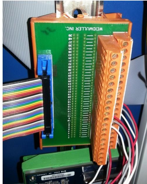
Figure 3-7: Intermediate board of SEL 421 relay
