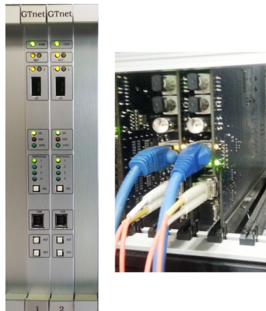
Figure 3-8: Front and back view of two GTNET cards
