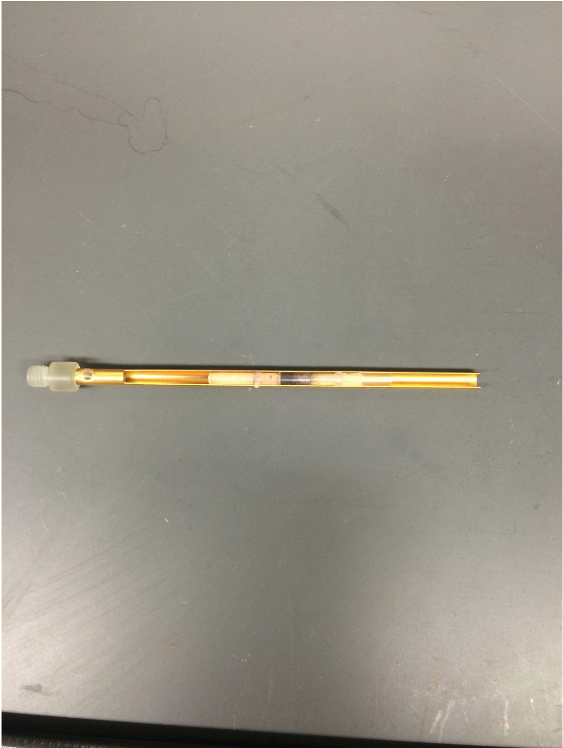
FIGURE 2.13: The material with known mass is placed inside a plastic holder and held at a fixed position in a brass clasp. The susceptibility of the holder and clasp are measured prior to measurement of the sample.
