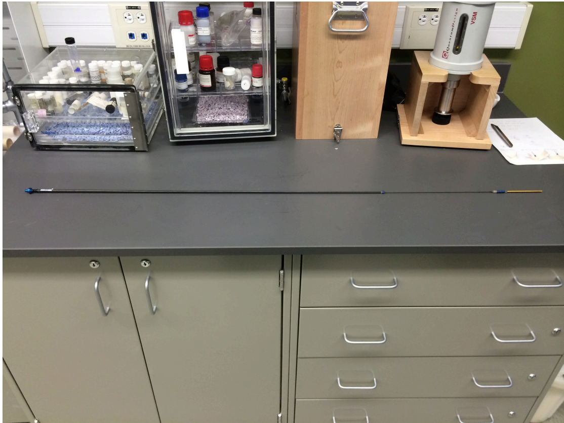
FIGURE 2.14: The brass holder is placed at the end of a long rod. This rod is vibrated inside a coil pickup at the bottom of the Physical Property Measurement System. The motor can be seen at the top right corner of the figure.
