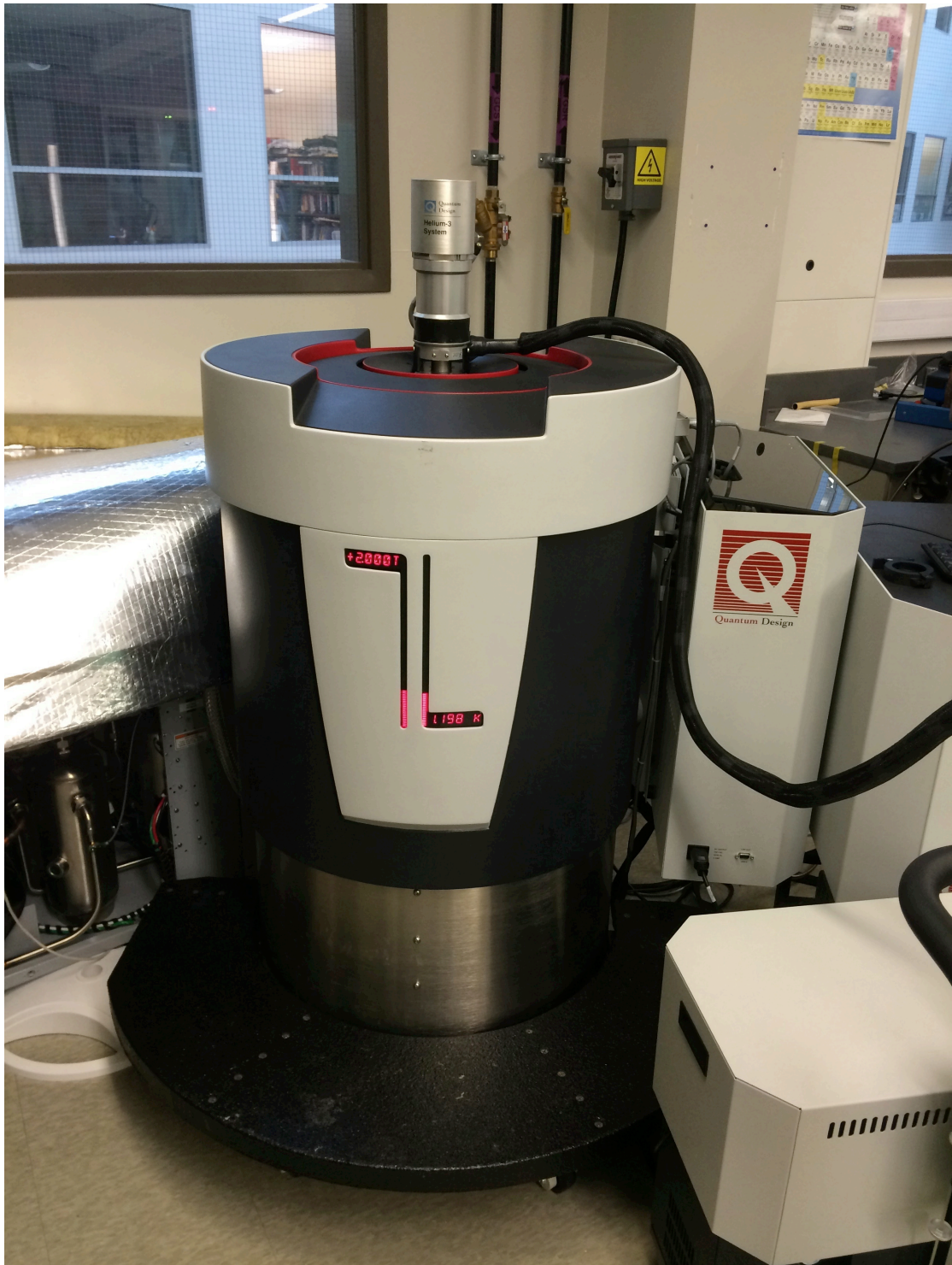
FIGURE 2.15: A superconducting ring can produce fields of up to 9 T at the base of the instrument. The sample rod is inserted through the top of the PPMS all the way to the base where the coil pickup sits.
