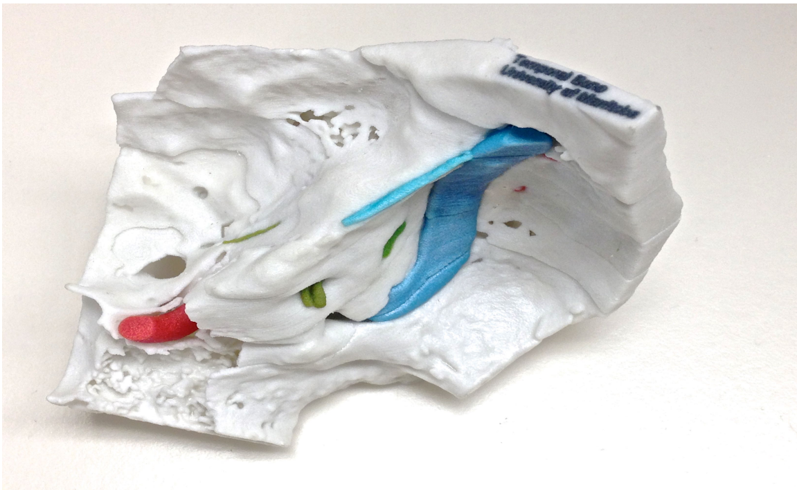
Figure 2 – Seen above is the rapid-prototyped printed bone model (PBM) that was used to assess surgical skill acquisition in novices for this study. It is derived from the same microCT data used in the virtual model (VM), and created using an in-house 3D Printing device. Note the colourization of the model, indicating vital structures.
