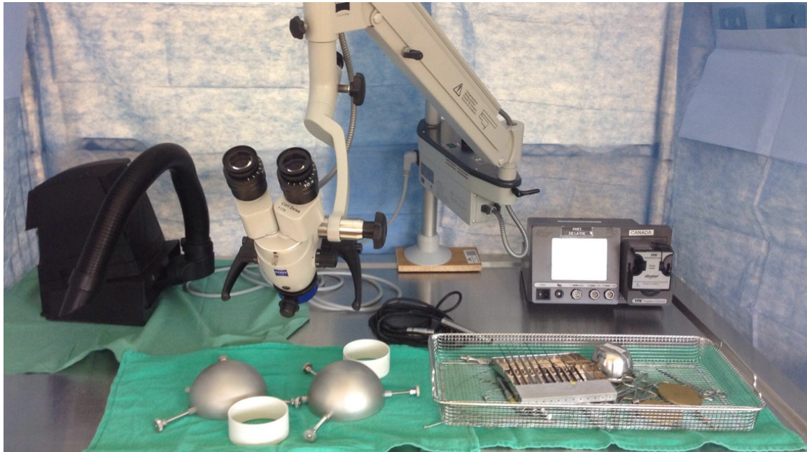
Figure 3 – The mock-surgery setup where participants performed the drilling of their printed bone model (PBM) specimens that were used in the grading and assessment of surgical ability for the study.
