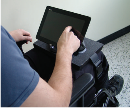
FIGURE 2: Tablet mounting platform for wheelchair use.
