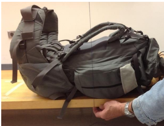
Figure 3.3: Using the reaction board technique to locate the centre of gravity of the backpack in the transverse plane.
