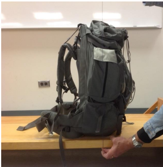
Figure 3.4: Using the reaction board technique to locate the centre of gravity of the backpack in the frontal plane.
