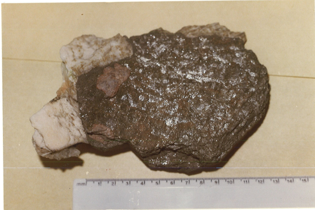
Figure 57(b). Planes of biotite + chlorite (reflecting light) showing parallel orientation.
