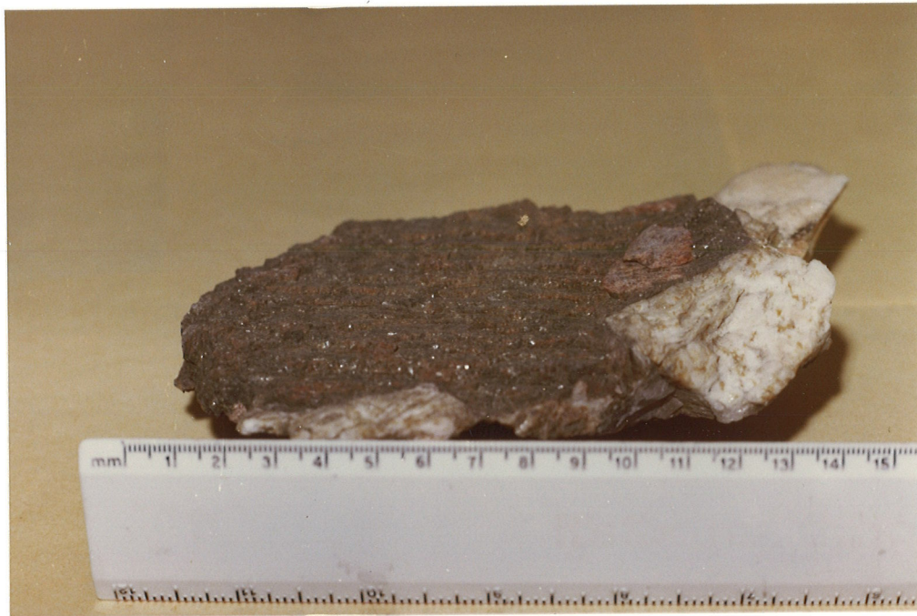
Figure 57(c). This parallel orientation of biotite + chlorite along cleavage planes which forms "layering" of the pseudomorph is shown as step-like boxwork sandwiching flattened garnet crystals.
