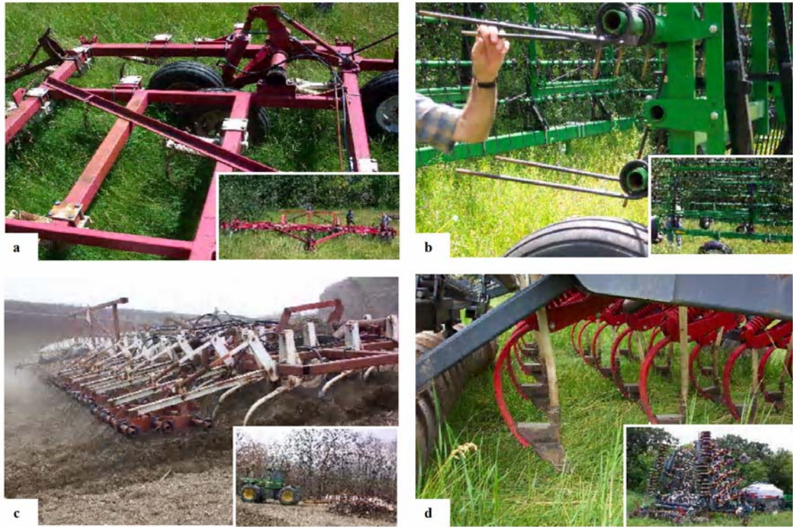
Figure 2.2 Photos of the four tillage implements: a) deep-tiller; b) spring-tooth-harrow; c) light-cultivator and d) air-seeder.
