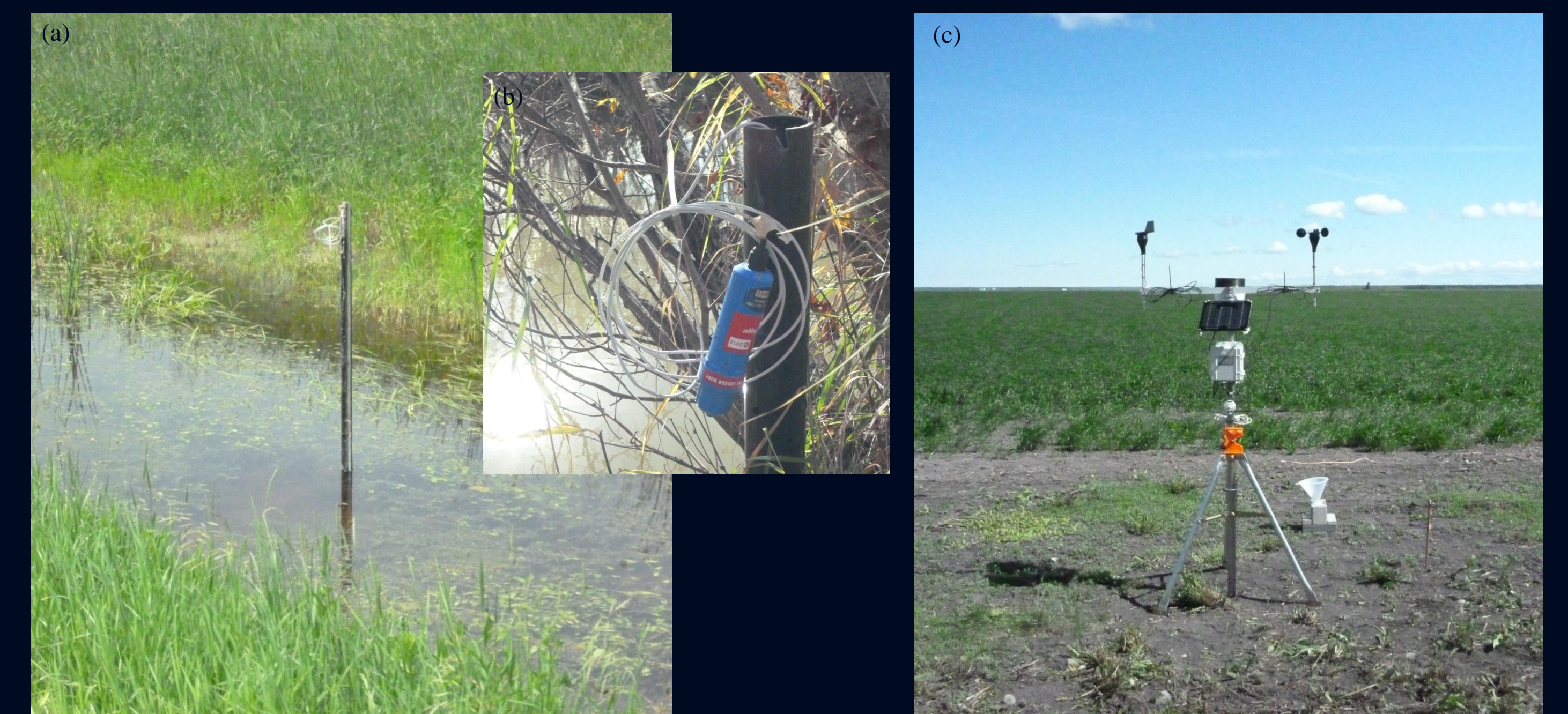
▲ FIGURE 2: (a) stilling well at Site 006; (b) Odyssey capacitance water level logger; and (c) HOBO U30 weather station;
