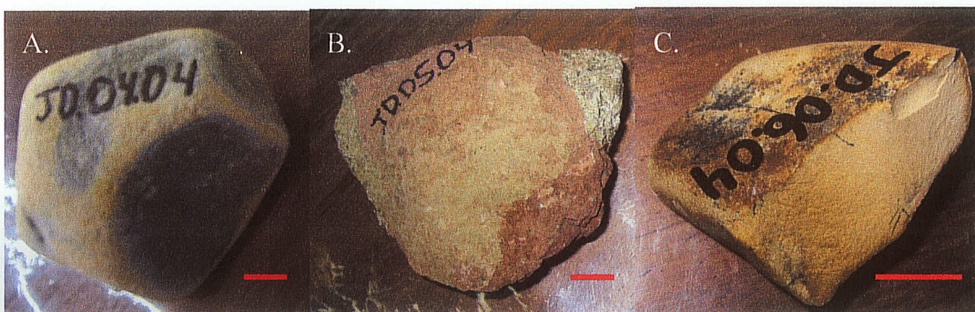
Figure 6.36: Chert samples from Punta Ple Del Gigante Beach, Nicaragua. (A.) Solid dark grey chert. (B.) Red nodule chert with inclusions. (C.) Bedded siliceous mudstone. Scale bar is 1 cm.
