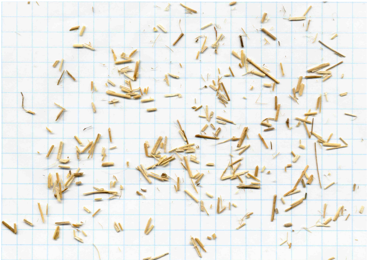
Figure 3.3 Example scan of flax shive sample for shape dimensions (grid = 1/4 inch).
