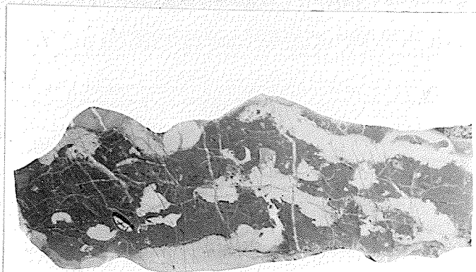
Figure 17. Etched surface showing "worm-like" structures. The light grey tubes consist of dolomite and the darker matrix consists of fine grained calcite. Near the top of the McKay group, north of Lamb Creek (magnification x 1).
