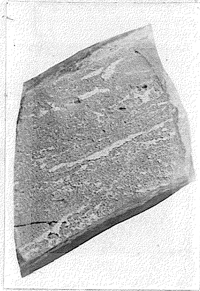
Figure 7. Etched surface showing coarse white dolomite crystals which form poorly defined laminae parallel to bedding in fine grained grey dolomite matrix. Upper Jubilee, Marmalade Creek section (magnification x 1).
