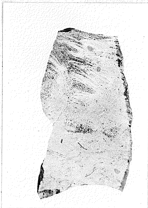
Figure 24. Etched surface showing Beaverfoot limestone with cross-bedded laminae of fine quartz sand. The sand, which is light colored and forms most of the mineral in this specimen, averages less than .1 mm. in diameter, and has authigenic overprints. The matrix which is darker colored consists of calcite. From the section at White Knight Mountain (magnification x 1).
