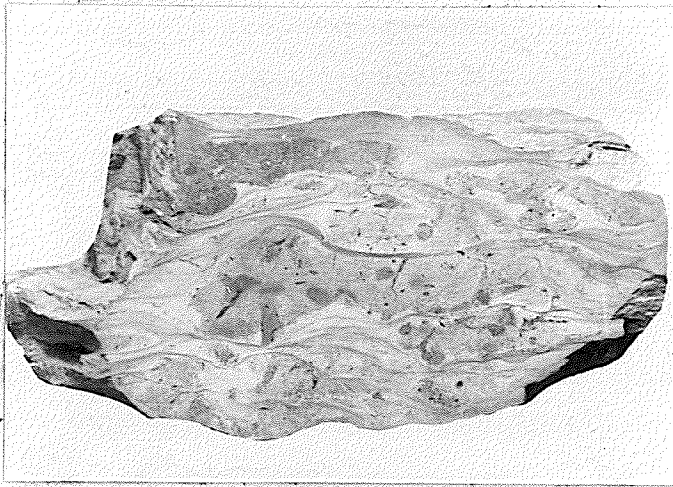
Figure 11. Etched surface of irregular nodular limestone. The thin dark wavy bands consist of argillaceous material and the lighter colored rock is limestone. The McKay group, Marmalade Creek (magnification x 1).
