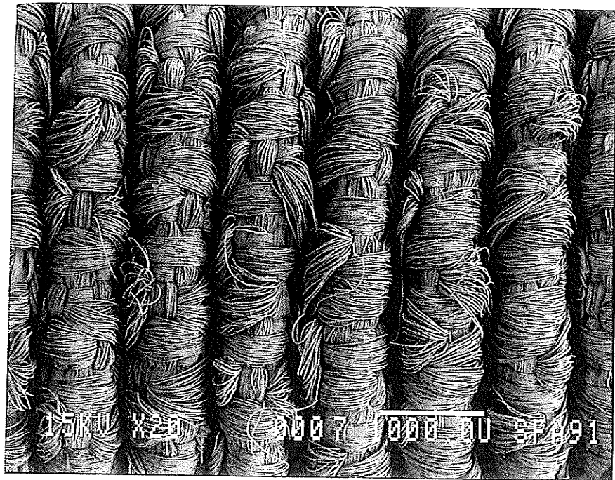
FIGURE 3E: SEM PHOTOMICROGRAPHS OF THE INTERNAL AND EXTERNAL SURFACES OF THE MEADOX WOVEN DOUBLE VELOUR PROSTHESIS.
