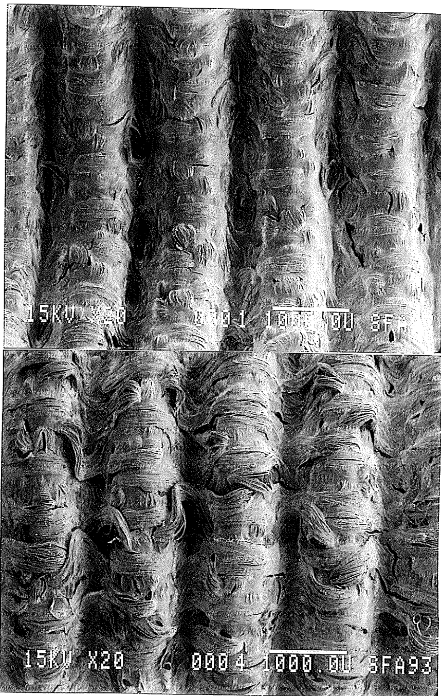
FIGURE 1E: SEM PHOTOMICROGRAPHS OF THE INTERNAL AND EXTERNAL SURFACES OF THE WOVEN HEMASHIELD®.
