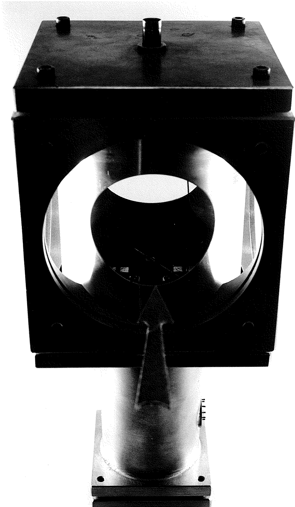
Fig. 4.2 Scanner and cylindrical pickup mounted in a standard beam cube.
