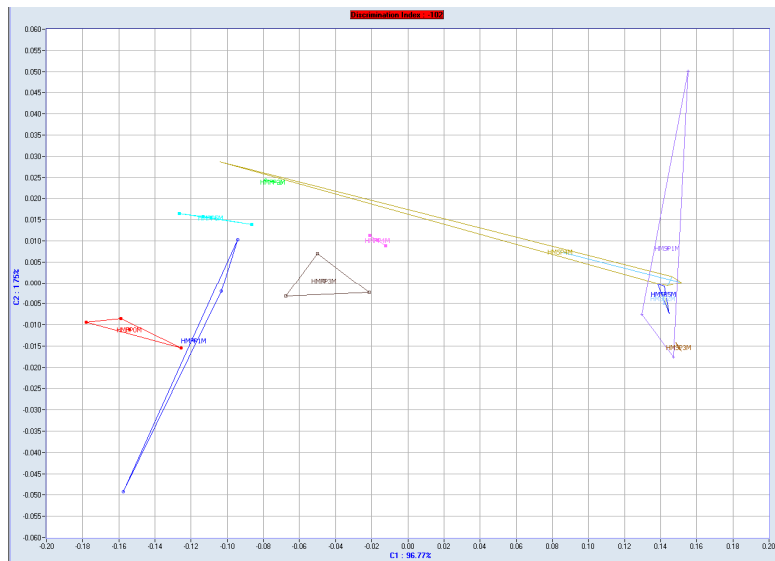
Figure app.5.20: PCA of the volatile compounds of pasteurized HM stored at -20^{\circ}\text{C} (FP) and at -80^{\circ}\text{C} (SP): pattern change during 5 months of storage
