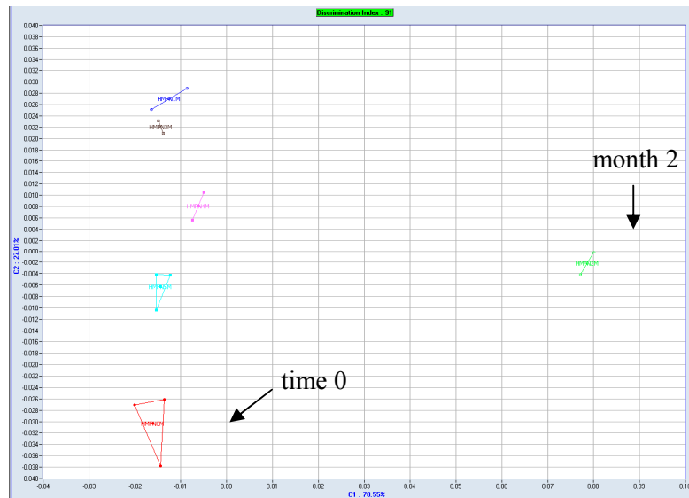
Figure 4.28: PCA of the volatile compounds of HM stored with nitrogen gas at -20°C (FN): pattern change during 5 months of storage
