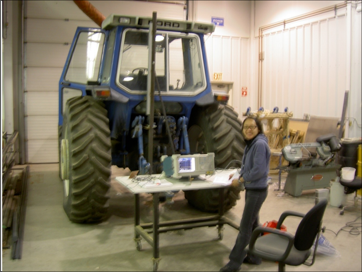
Fig. 4.6 A snapshot of the noise acquisition setup.
