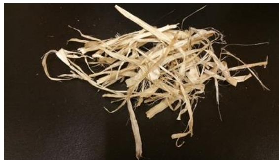
Figure 3.6. Virgin water-retted Brassica napus fibres at the University of Manitoba in 2014.
