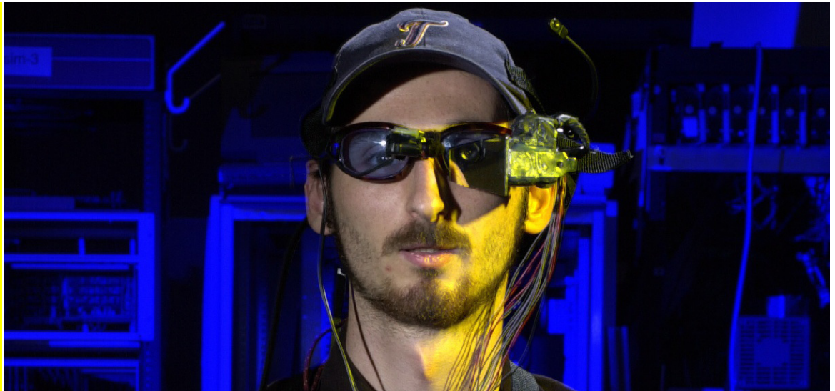
Figures 63 - Image of Steven Mann's EyeTap, a device that allows for the capture and augmentation of data using the natural functioning of the eye.
