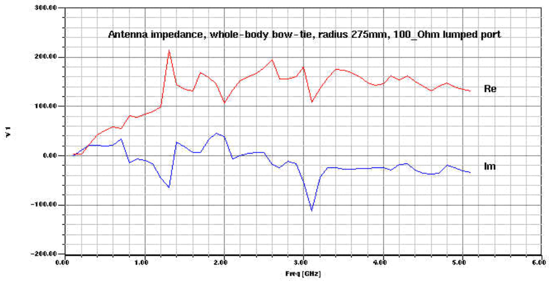
Figure 5.6 Simulation result of antenna impedance of whole-body bow-tie
