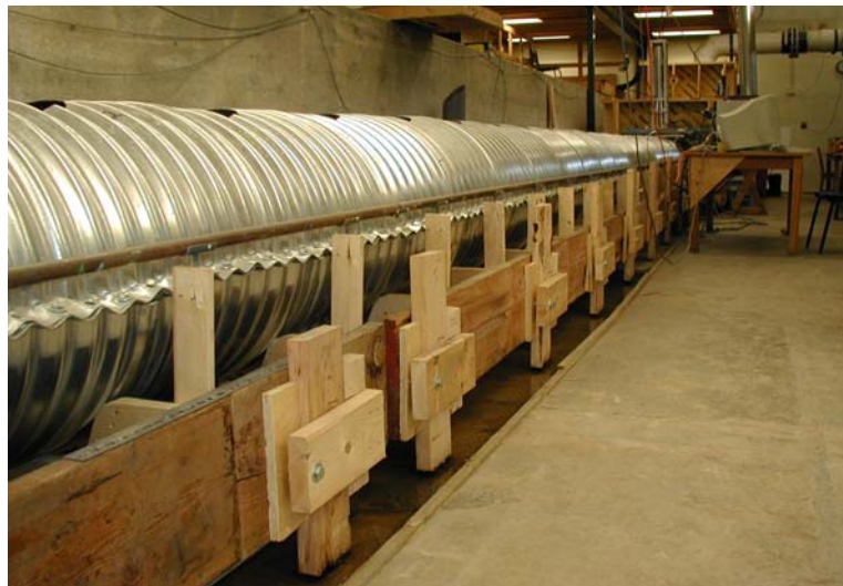
Figure 3.10: View facing upstream of culvert and supports (set at 0% slope).
