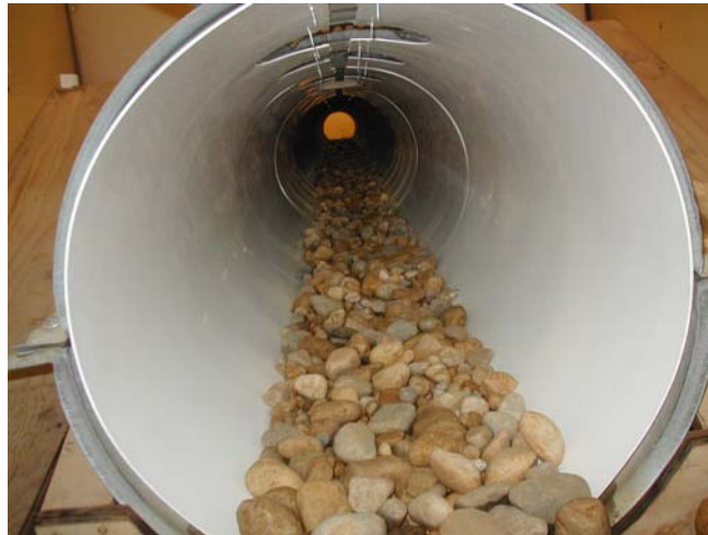
Figure 4.2: View of culvert looking downstream from the inlet with smooth-walled insert installed in the first six cross-sections.
