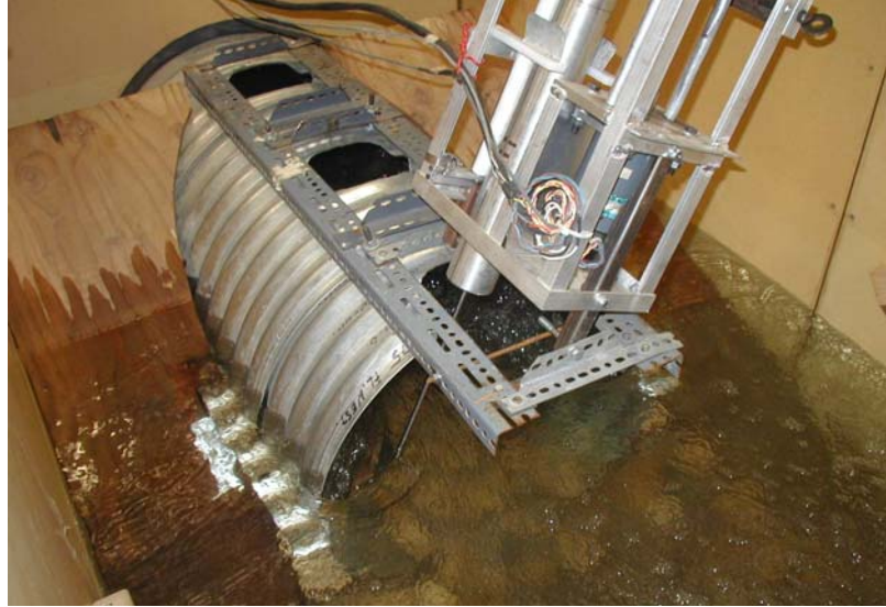
Figure 3.18: Mast set up at cross-section 1 and angled to allow the ADV to sample the left side of the cross-section.
