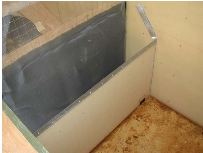
Figure 3.5: Sharp crested weir showing nappe splitters used for aeration demand.
