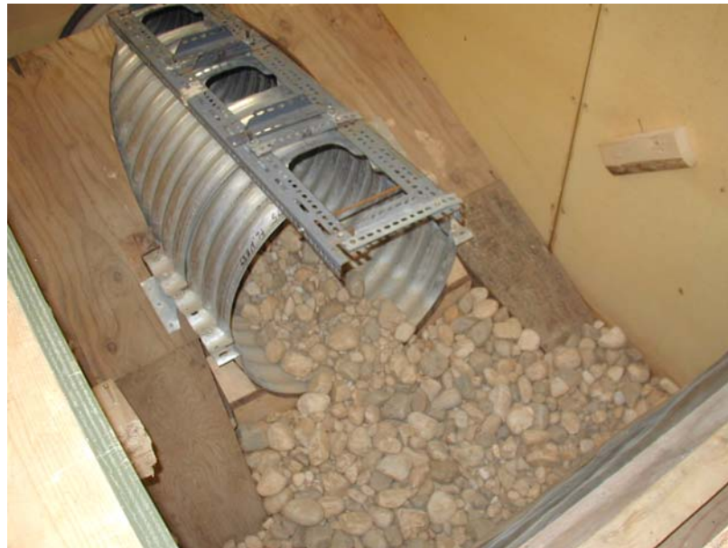
Figure 3.4: Projecting inlet showing simulated road embankment and gravel bed.
