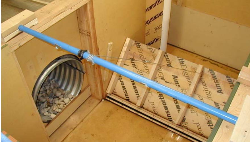
Figure 3.11: Layout of culvert outlet, tailwater gate and tailwater box outlet.
