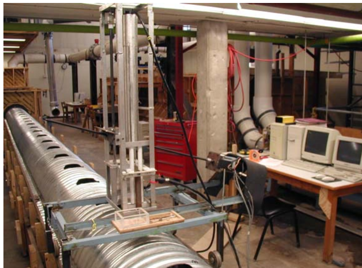
Figure 3.17: Automated sampling system showing the sampling cart, control computers and sampling mast with ADV in fully withdrawn position (ADV is not visible).
