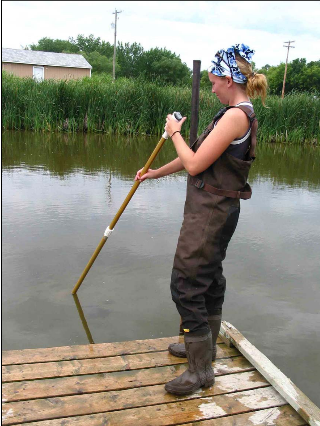
Figure 3.6 Photograph of the Global Water FP101 flow probe used to take flow measurements at sample sites.
