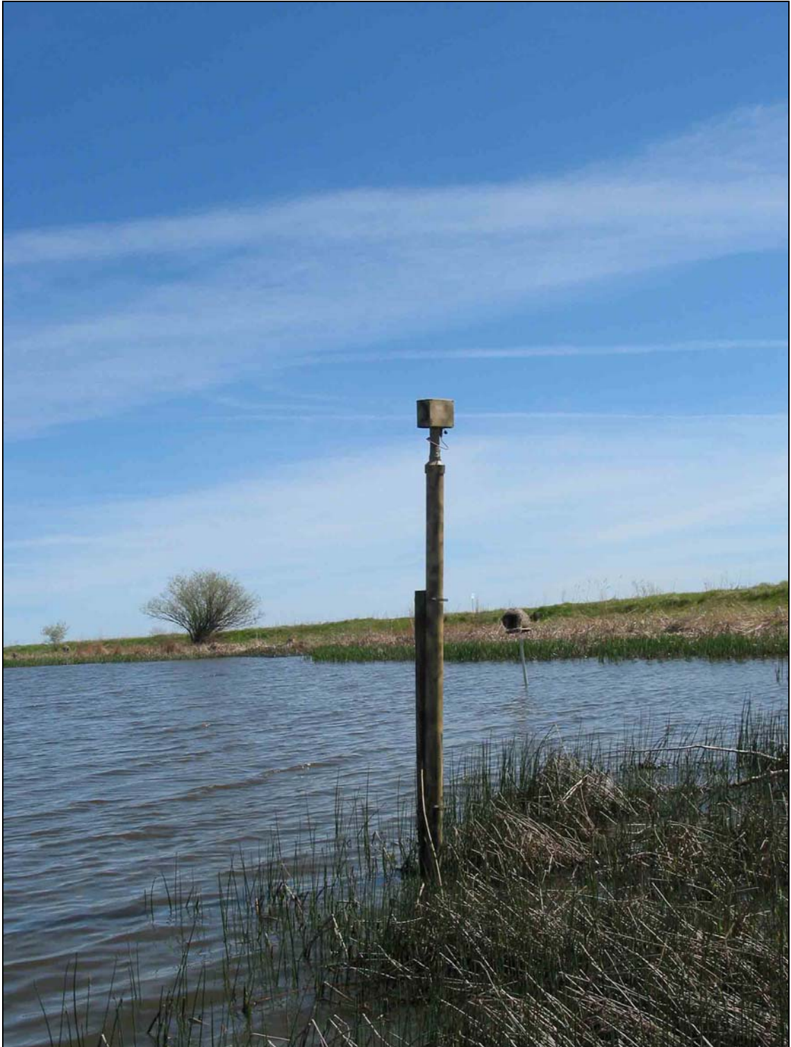
Figure 3.4 Photograph of the water level monitor deployed at site 7 at Portage Creek South (PCS) in 2005.
