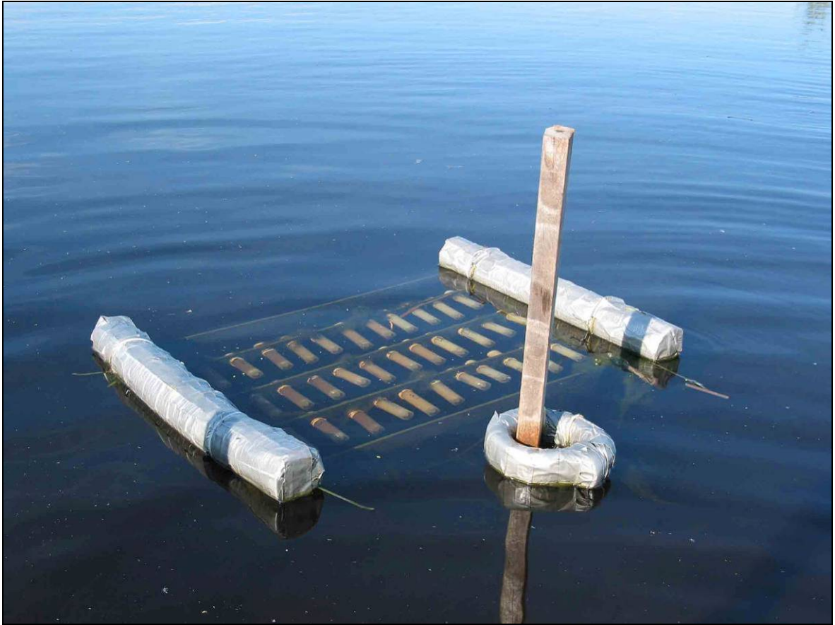
Figure 3.17 Picture of frame containing NDS anchored at sample site in Canvasback Bay in 2002. A circular float attached the frame to the stake, allowing the frame to move freely around the stake with changes in current direction.
