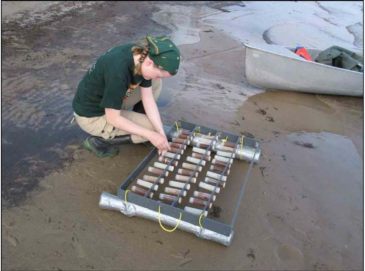
Figure 3.16 Picture of NDS vials being attached to a PVC frame.
