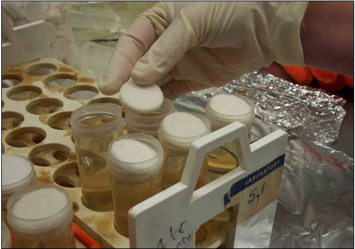
Figure 3.14 Preparation of NDS vials in laboratory. Silica frits are being added to vials containing warm agar solution.
