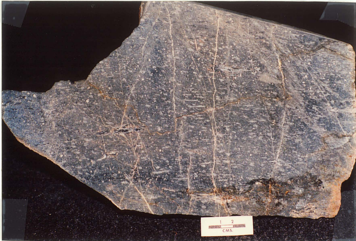
Figure 18: Slab of quartz-plagioclase-phyric felsic flow that has been etched with hydrofluoric acid. The abundant creamy, oval to elongate features are recrystallized quartz crystals. The small white spots are recrystallized feldspar crystals, composed of epidote, clinozoisite, carbonate, zoisite, and local remnants of plagioclase.
