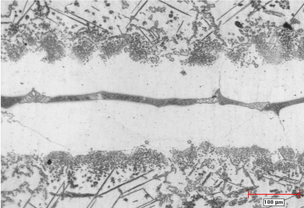
Figure 4.3: Micrograph of IN738 bonded with 76 \mu\text{m} MBF80 filler at 1180 ^{\circ}\text{C} for 7 hrs (X200)
