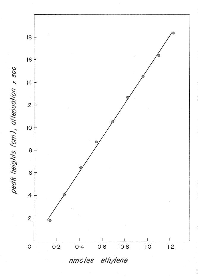
Fig. 2. Standard curve for ethylene at medium concentration ranges.
