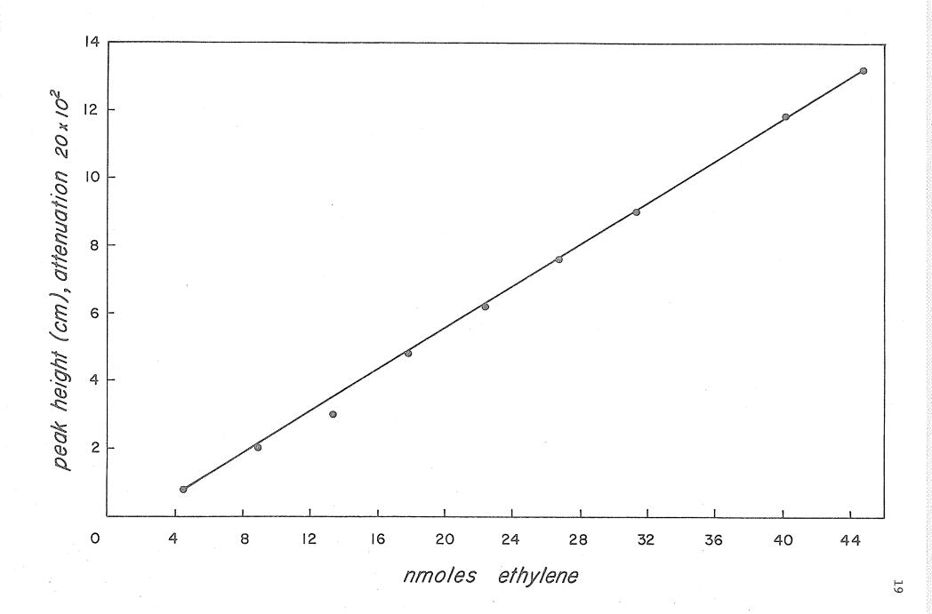
Fig. 3. Standard curve for ethylene at high concentration ranges.
