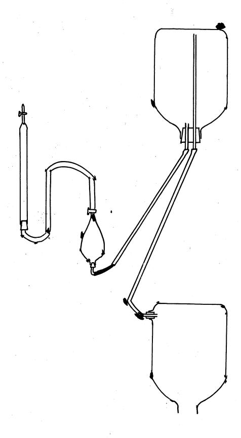
top and connected to bottle "B" on the table. Bottle "B" has an inlet from "A" and an outlet leading to the reservoir. As water flows from "A" to "B" under the force of gravity the air in "B" is compressed which transfers the pressure through the buffer in the reservoir, to the column.
