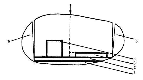
Figure 7. Original location in the tuber of samples used in different tests; B- bud end, S- stem end, 1- discarded slice, 2- tensile test specimen, 3- small strain dynamic shear test specimen, 4- wedge-penetration fracture test specimen.
