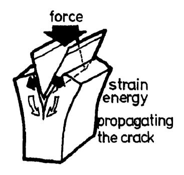
Figure 3. Diagram representing the propagation of the crack in the wedge fracture test. The black arrows on the specimen represent the force which is transmitted from the wedge to the two 'halves' of the specimen, forcing them apart such that they store strain energy. The white arrows refer to the stored strain energy which can be fed to the advancing crack once the failure stress has been reached. (Adapted from Vincent, 1990)
