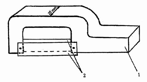
Figure 9. The cutting device ('cuber') used to take samples for the wedge-penetration fracture test; 1- plastic handle, 2- metallic blades.
