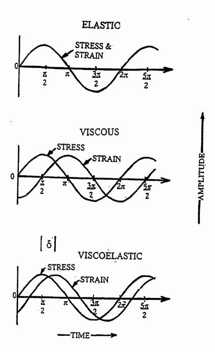
Figure 5. Stresses and strains of elastic, viscous and viscoelastic bodies subjected to dynamic tests by a controlled stress rheometer (Adapted from Pang, 1995)
