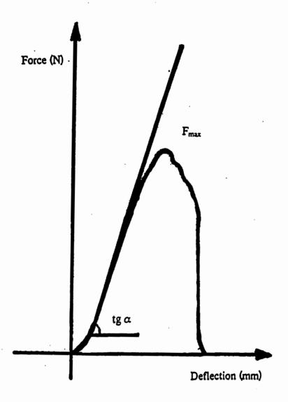
Figure 10. Typical force-deflection curve obtained in the tensile test.
