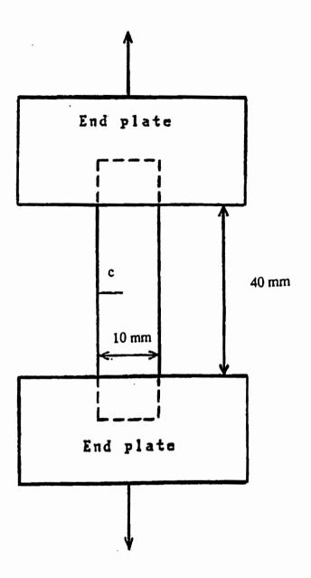
Figure 8. Dimensions and experimental set-up of potato specimen used in tensile test (Adapted from Fahloul and Scanlon, 1996).
