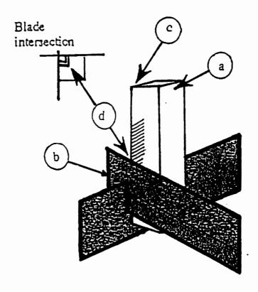
Figure 6. Graphical representation of the feathering phenomenon as it occurs on the potato strip at the intersection of two blades; (a) cut potato strip; (b) blade intersection; (c) strip corner where most friction exists; (d) feathering (Adapted from Anonymous, 1998).
