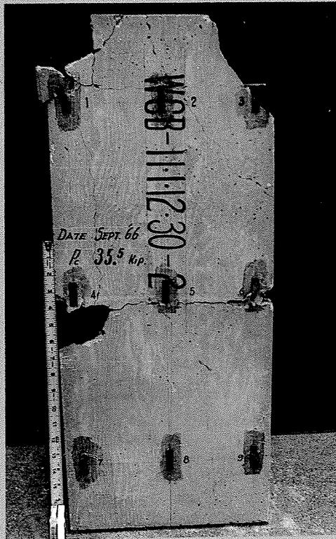
PLATE No. 11. View of Panel WCB 11.1.12.30- 2 after Failure.
