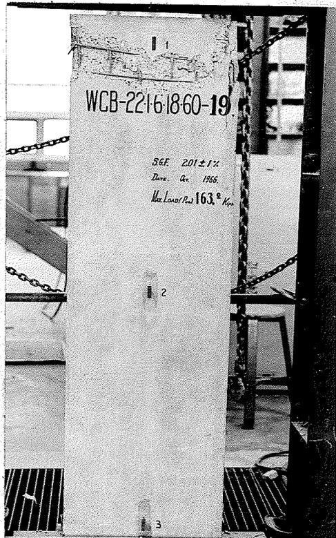
PLATE No. 28. Front View of WCB 22.1.6.18.60- 19 after Failure.
