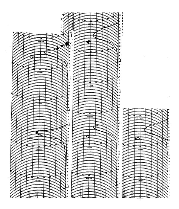
Figure 28. Extensigrams for composite flours containing increasing proportions of maize oil:
