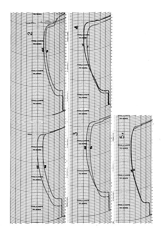
Figure 29. Farinograms for composite flours containing increasing proportions of maize oil:
