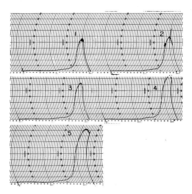
Figure 22. Extensigrams for composite flours containing increasing proportions of maize protein isolate:
