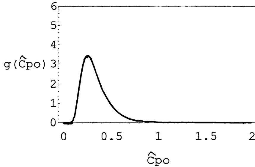
Figure 3.2.2.2b Density of  $\hat{C}_{po}$  with  $a'\theta = .5$ ,  $n = 10$ ,  $r = 2$ , and  $s = 9$ .
