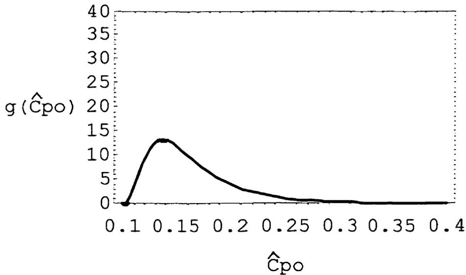
Figure 3.2.1.2b Density of  $\hat{C}_{po}$  with  $a' = .1$ ,  $n = 10$ ,  $r = 2$  and  $s = 9$ .
