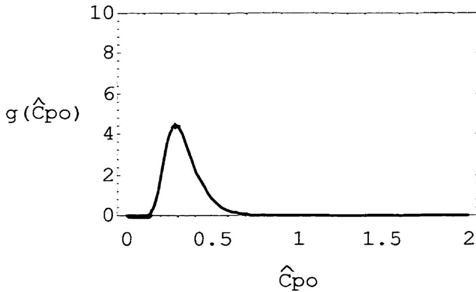
Figure 3.2.2.3b Density of  $\hat{C}_{po}$  with  $a'\theta = .5$ ,  $n = 20$ ,  $r = 3$ , and  $s = 17$ .
