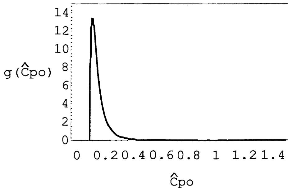
Figure 3.2.1.1a Density of  $\hat{C}_{po}$  with  $a' = .1$ ,  $n = 5$ ,  $r = 1$  and  $s = 5$ .
