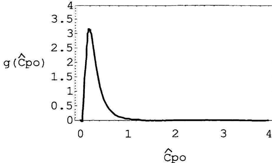
Figure 3.2.2.1a Density of  $\hat{C}_{po}$  with  $a'\theta = .5$ ,  $n = 5$ ,  $r = 1$ , and  $s = 5$ .
