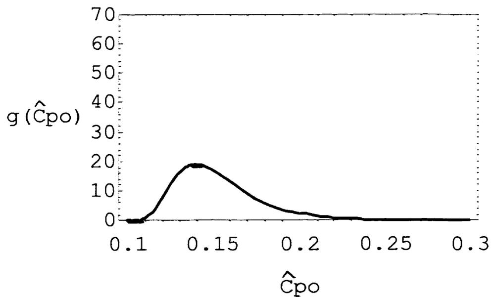
Figure 3.2.1.3b Density of  $\hat{C}_{po}$  with  $a' = .1$ ,  $n = 20$ ,  $r = 3$  and  $s = 17$ .
