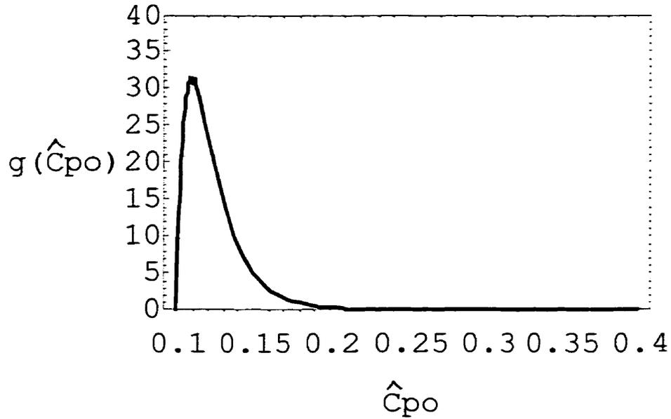
Figure 3.2.1.2a Density of  $\hat{C}_{po}$  with  $a' = .1$ ,  $n = 10$ ,  $r = 1$  and  $s = 10$ .
