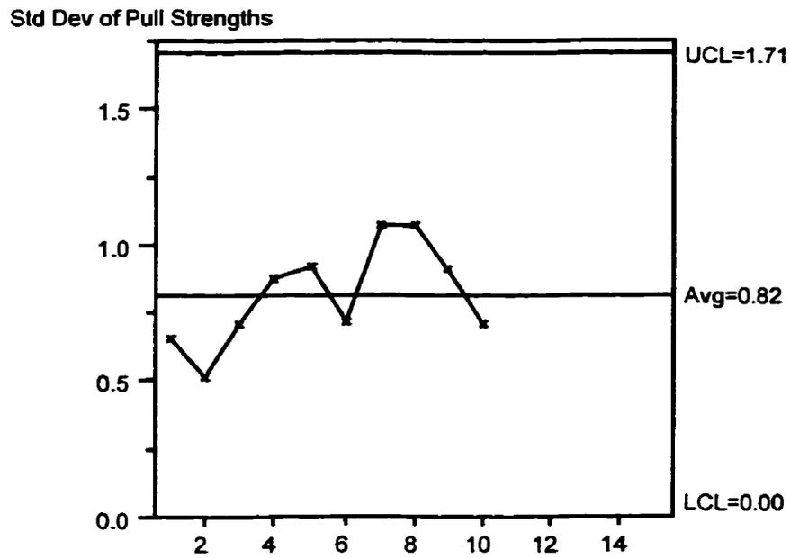
Figure 2.6.2  $\bar{x}$  and s chart of Adjusted Breaking Strengths
