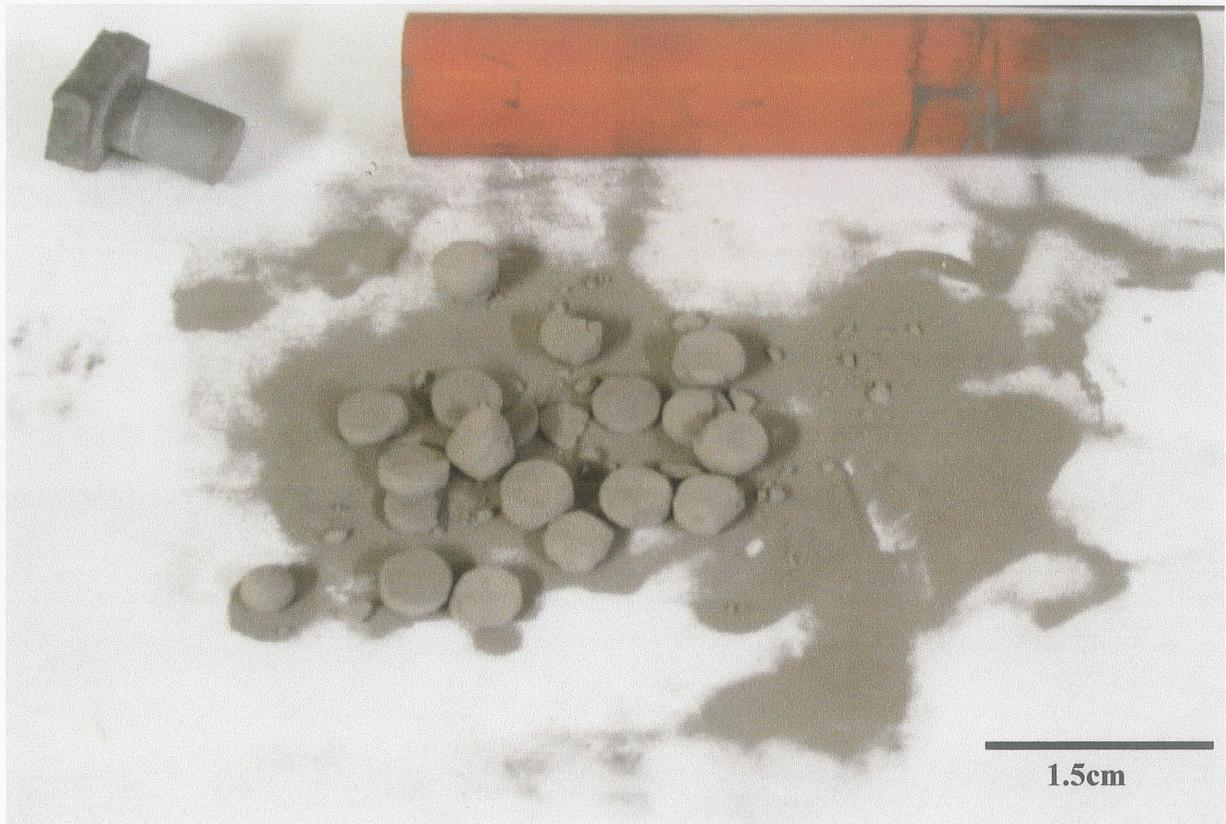
Figure 4.10: Picture showing cold isostatically pressed powder
