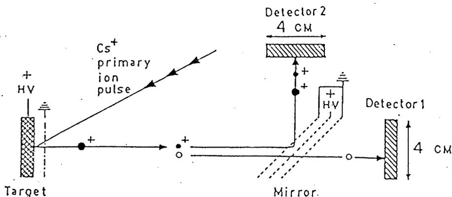
Figure 1.4. Instrumental arrangement for the analysis of positive ions
