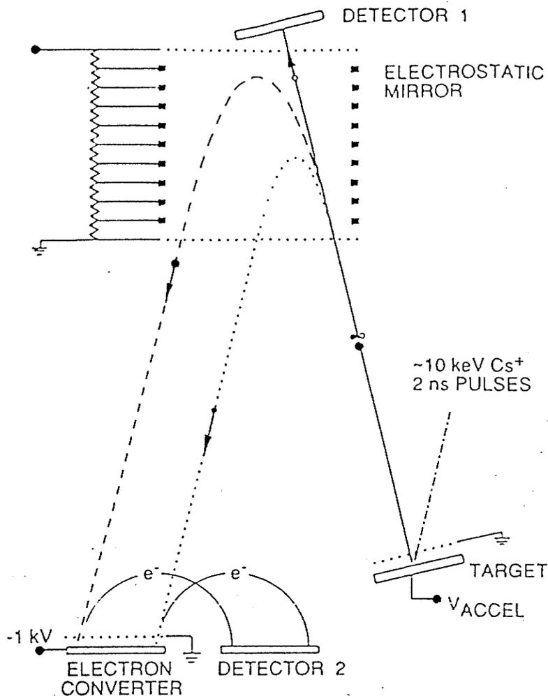
Figure 1.5. Schematic diagram of the Manitoba TOF II mass spectrometer
