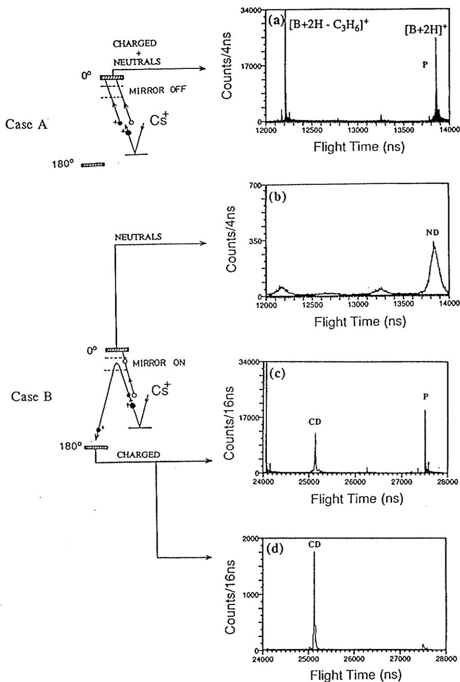
FIGURE 4.2 Analysis of ion decompositions in field-free flight. (a) Part of direct positive spectrum of ip<sup>4</sup>dT recorded with the ion mirror "off". (b-d) Spectra recorded with mirror "on": (b) neutral daughters (ND) of [B + 2H]<sup>+</sup>; (c) reflected parent (P) and charged daughter (CD) ions; (d) reflected CDs correlated with NDs.
