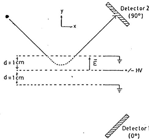
An ion trajectory in the electrostatic mirror; E is greater than the minimum value required to deflect the ion into detector 2
