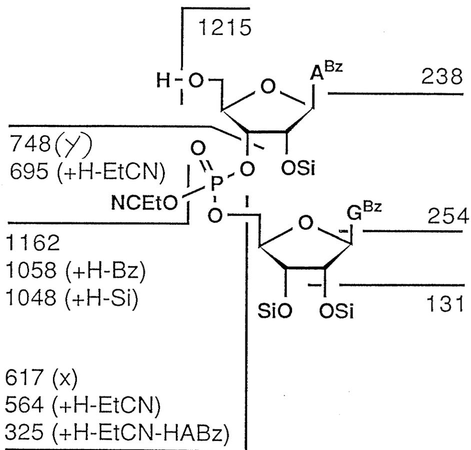
Figure 5.2 Some important fragments observed in the negative ion TOF-SI mass spectrum of ApG
