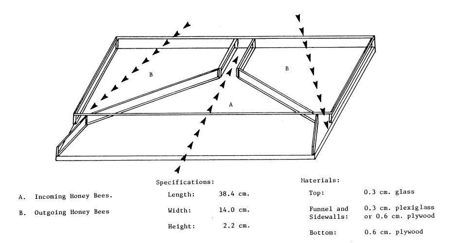
FIGURE 5. Two-way entrance device in place.
