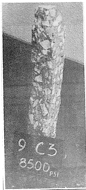
Typical vertical split failure of a high strength test cylinder.
