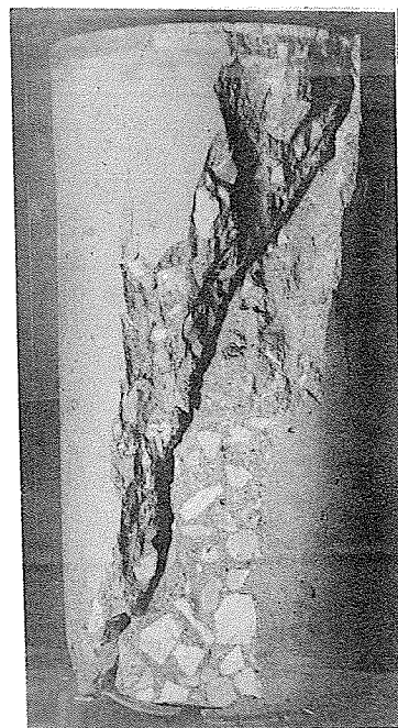
Diagonal shear failure.
