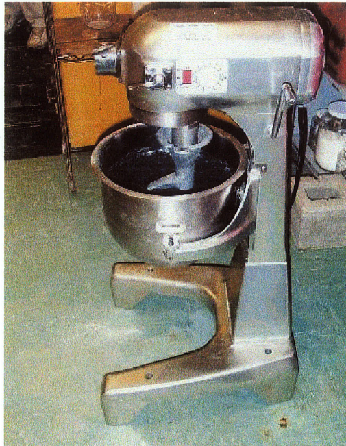
Figure 6: The Hobart mixer that was used to mix the biosolids with the lime and or PAM.
