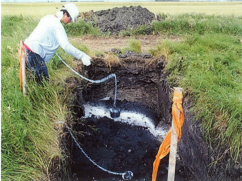
Figure 4: Cages loaded with the mixed product and the Ascaris suum ova and reovirus packets are deposited into the trench partially filled with the mixed product.
