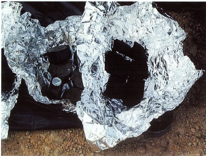
Figure 1: Sentinel chambers containing Ascaris suum ova on the left and garden cloth packets containing reovirus on the right.
