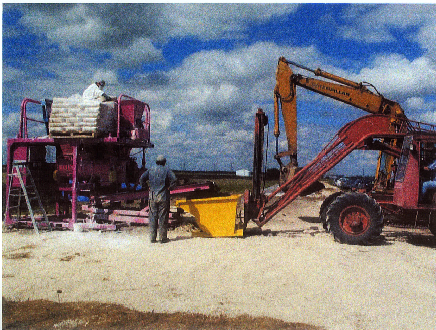
Figure 2: The Lodige sludge mixer set up at the WEWPCC.
