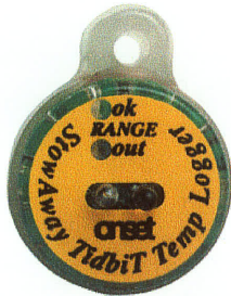
Figure 7: StowAway Tidbit Temp Loggers™ that was buried in the biosolids to record temperature (Onset Computer Corporation, 1996).
