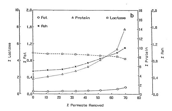
Figure 12. Changes in flux rate and solids (a) and composition (b) of skim milk during diafiltration through a diaflow hollow fiber membrane (10,000 m.w. cut off).
