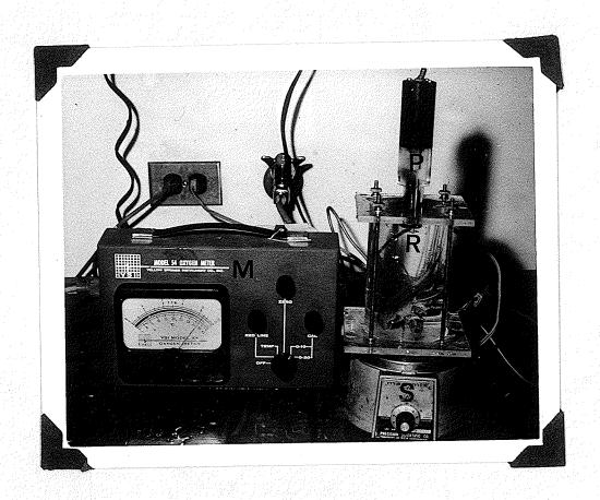
Oxygen concentration was measured at the beginning of the trial and after 3 minutes on the stirrer. The difference was recorded as the oxygen consumption under active metabolic conditions.
