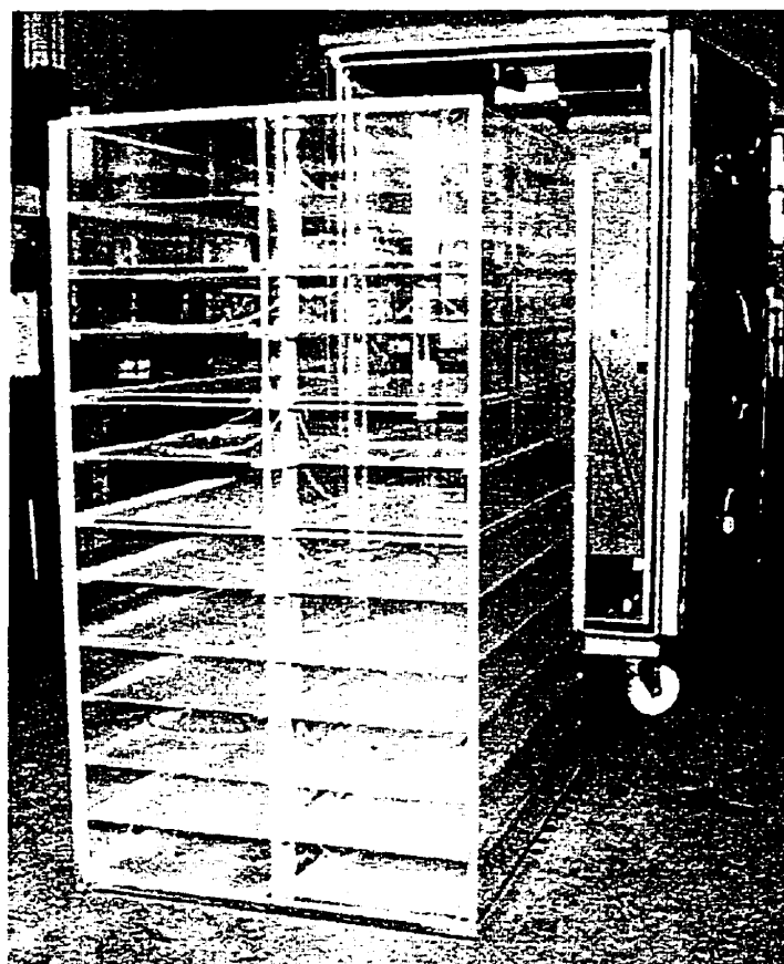
Fig. A.11. Removing the acrylic door which is fitted to the acrylic box by magnetic seal.
