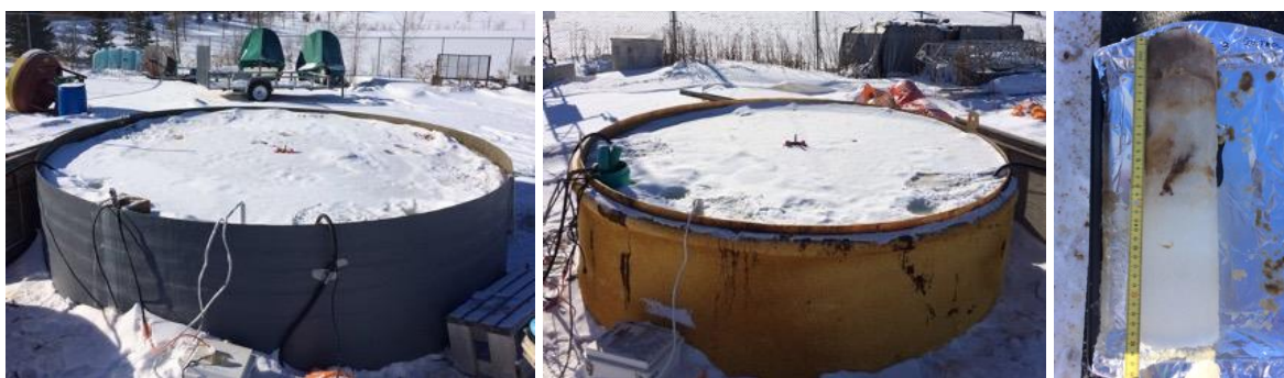
Fig. 4.1 Augmented tank (left), Native tank (middle), and an example of an ice core taken during the experiment (right). Photos were taken Feb. 26/18.
