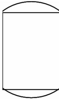
Fig. 5.2: Cleaved wafer with top and bottom intact to prevent shorting of top and bottom metal deposited in subsequent sputter deposition steps.
