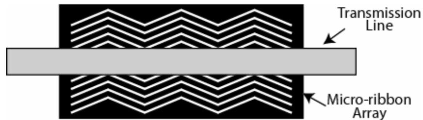
Fig. 1.4: Top view of the phase shifter showing the orientation of the transmission line over micro-ribbons.
