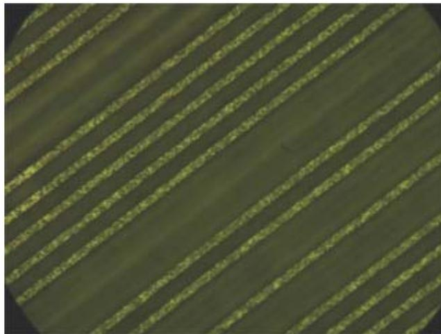
Fig. 5.13: Photograph of 10  $\mu\text{m}$  wide micro-ribbons with 10  $\mu\text{m}$  spacing. Released ribbons are out of plane and no longer in focus.
