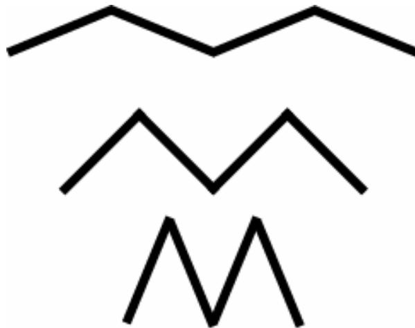
Fig. 4.10: Illustration of the 4-segment geometries at  $22.5^\circ$ ,  $45^\circ$ , and  $67.5^\circ$  with each segment being  $500\ \mu\text{m}$  in length.
