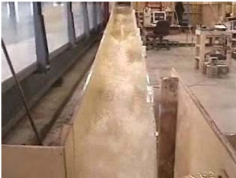
**Figure 4.13** Shock waves at skimming flow regime. a) Model II. b) Model III.
