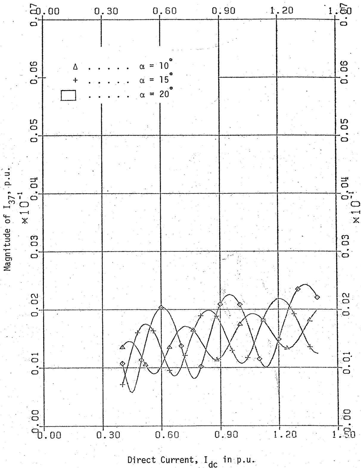
Fig. 2.14 Magnitude of 37th harmonic current as a function of  $I_{dc}$  in SB connection.
