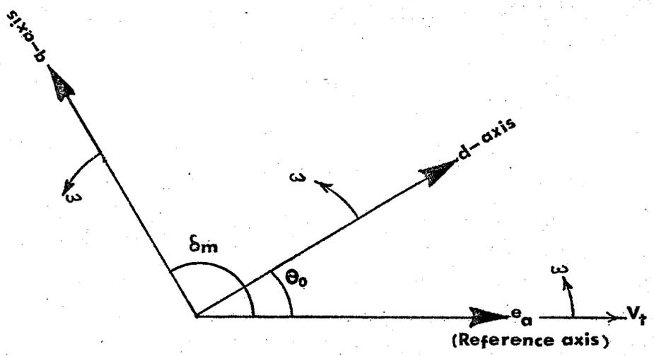
Fig 3-1 Position of rotor d-axis at  $t=0$
