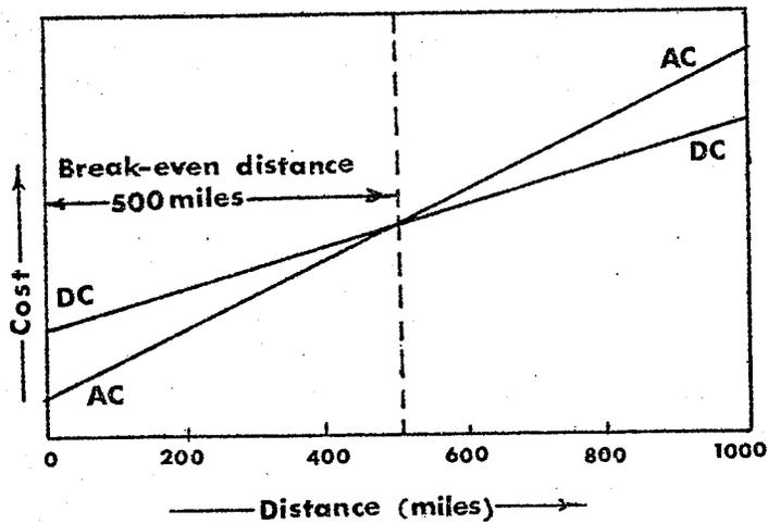
Fig 1.1 Comparative costs of ac and dc overhead lines versus distance
