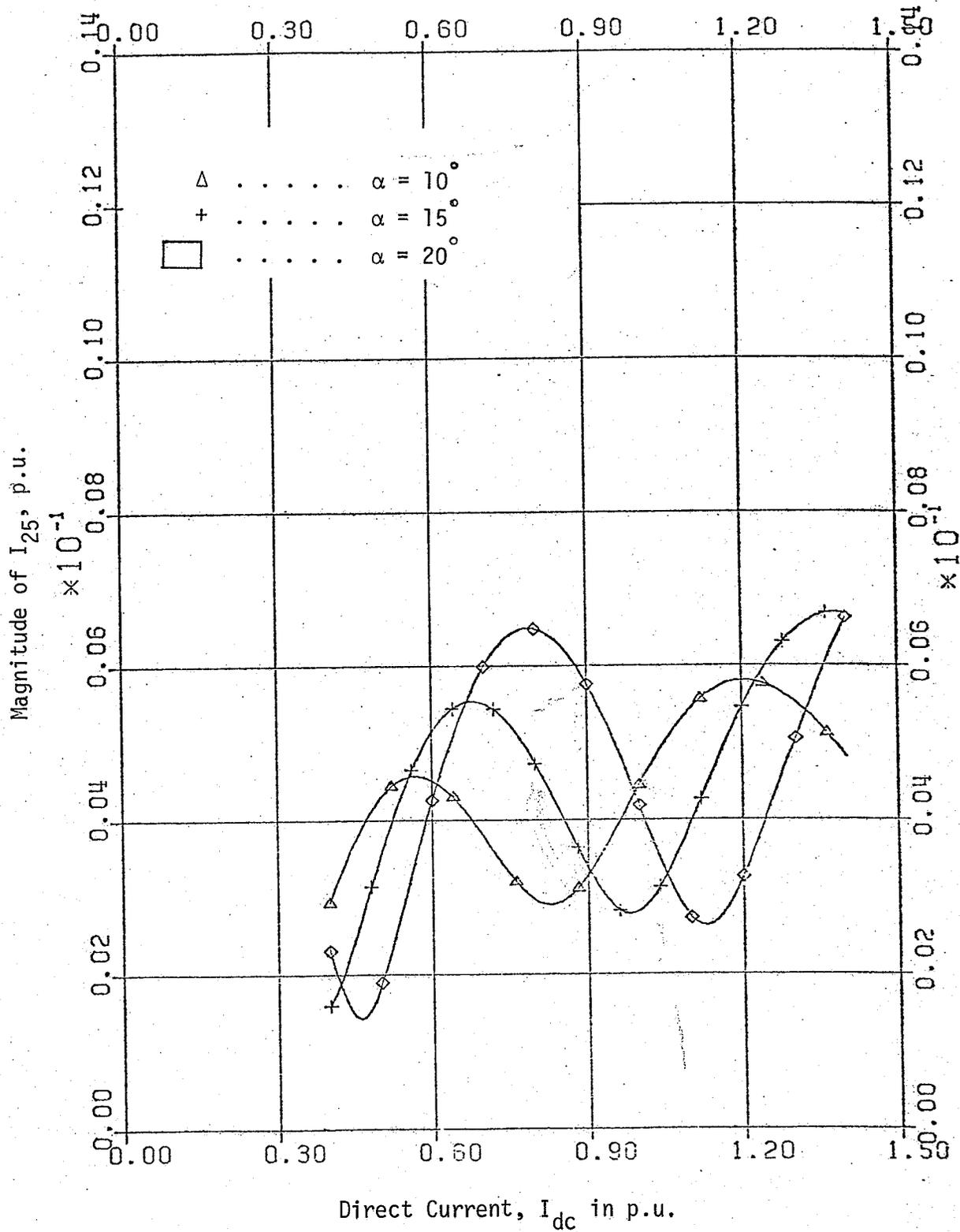
Fig. 2.18 Magnitude of 25th harmonic current as a function of  $I_{dc}$  in  $\Delta$  connection.
