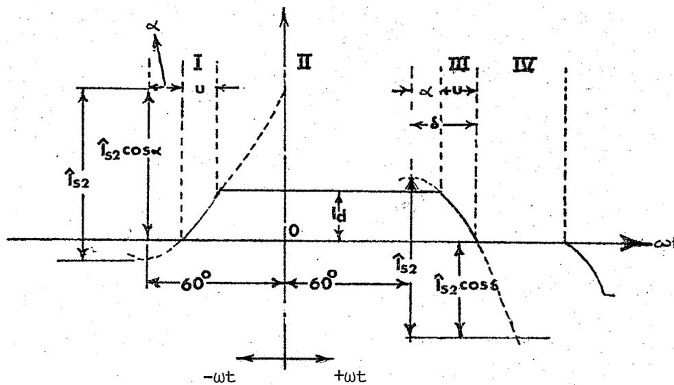
Fig 2-2 (b) Current in phase a
