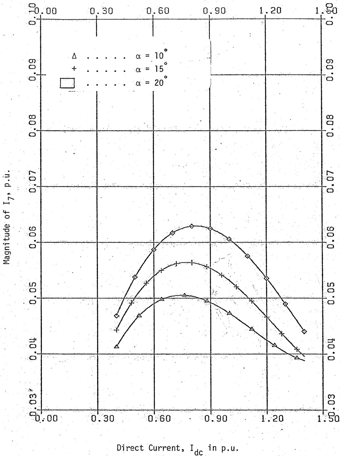
Fig. 2.4 Magnitude of 7th harmonic current as a function of  $I_{dc}$  in SB connection.
