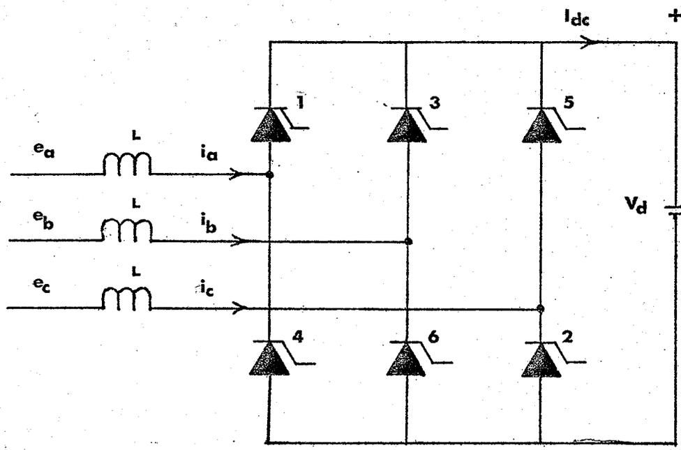
Fig 2-1 Bridge-Connected Rectifier
