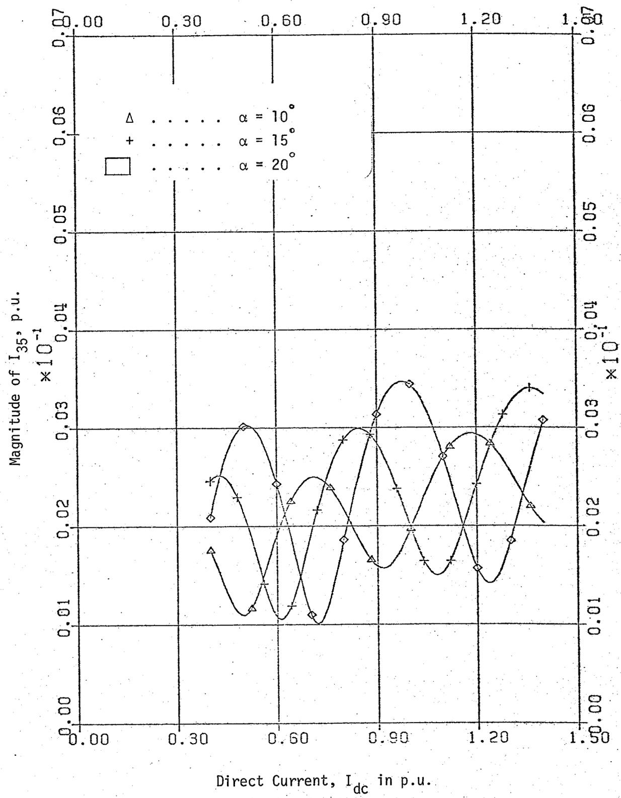
Fig. 2.19 Magnitude of 35th harmonic current as a function of  $I_{dc}$  in DB connection.
