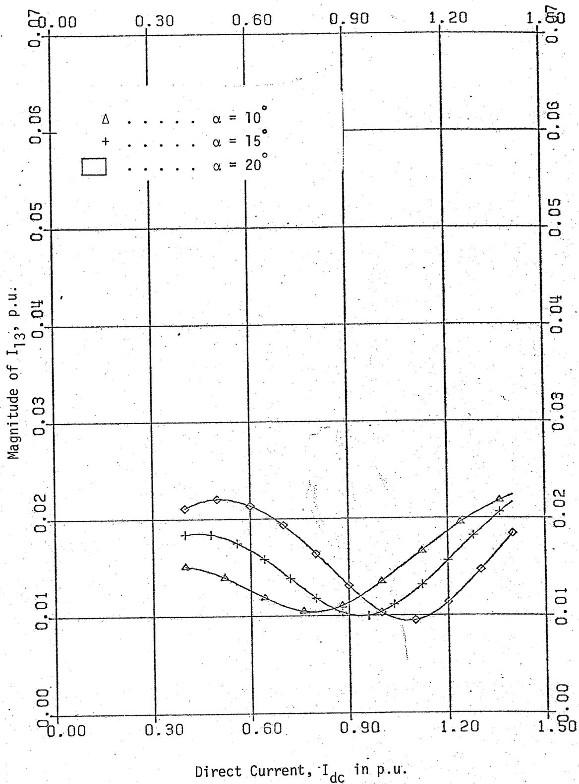
Fig. 2.16 Magnitude of 13th harmonic current as a function of  $I_{dc}$  in DB connection.
