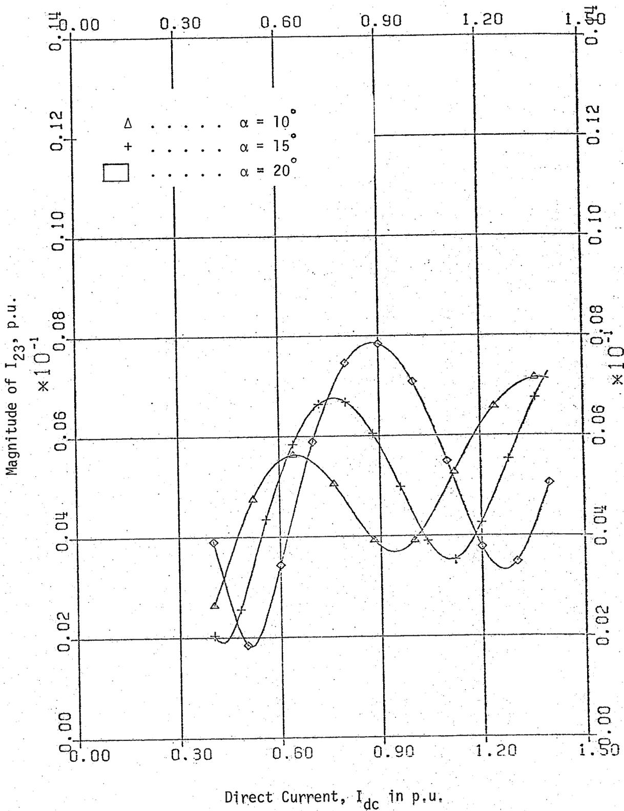
Fig. 2.17 Magnitude of 23rd harmonic current as a function of  $I_{dc}$  in DB connection.
