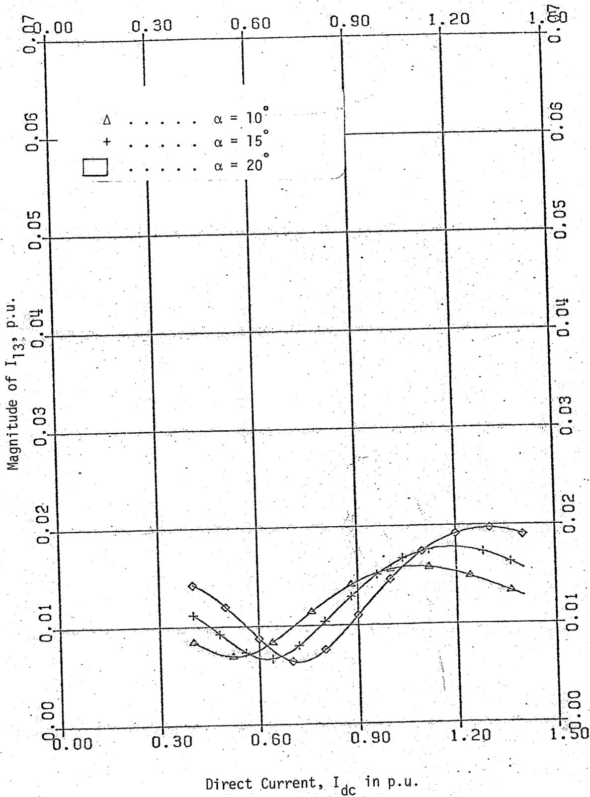
Fig. 2.6 Magnitude of 13th harmonic current as a function of  $I_{dc}$  in SB connection.
