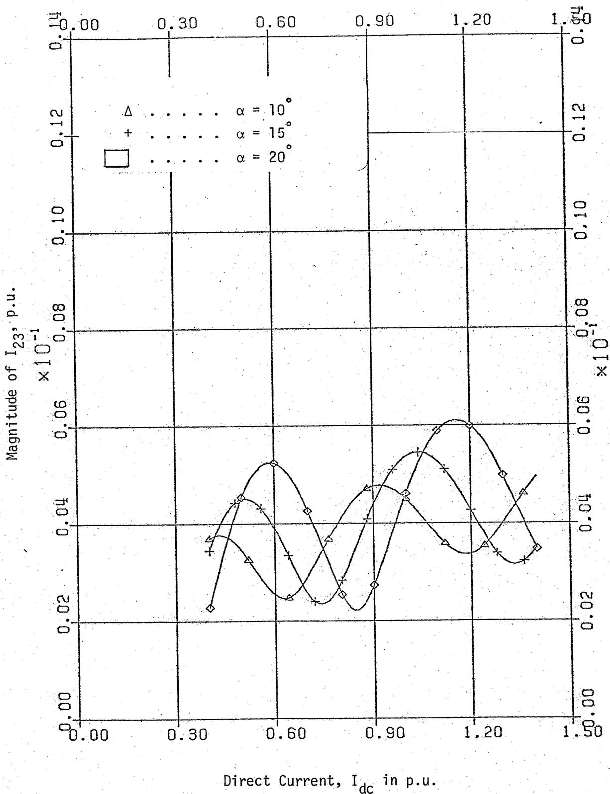
Fig. 2.9 Magnitude of 23rd harmonic current as a function of  $I_{dc}$  in SB connection.
