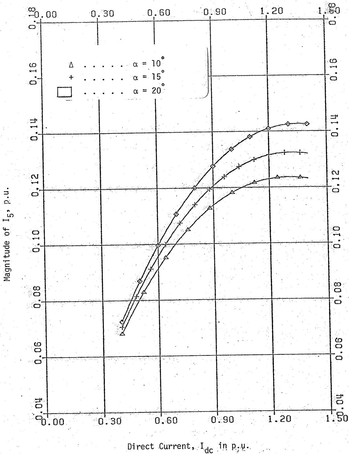
Fig. 2.3 Magnitude of 5th harmonic current as a function of  $I_{dc}$  in SB connection.
