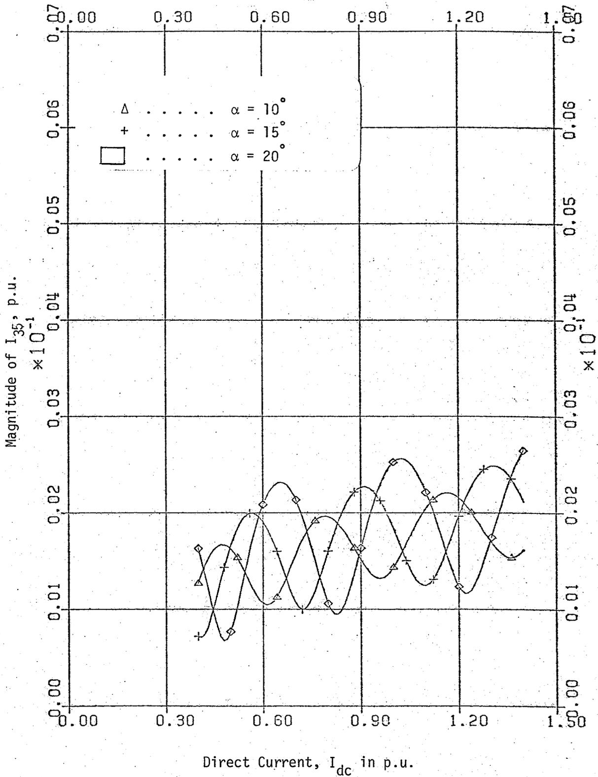
Fig. 2.13 Magnitude of 35th harmonic current as a function of  $I_{dc}$  in SB connection.
