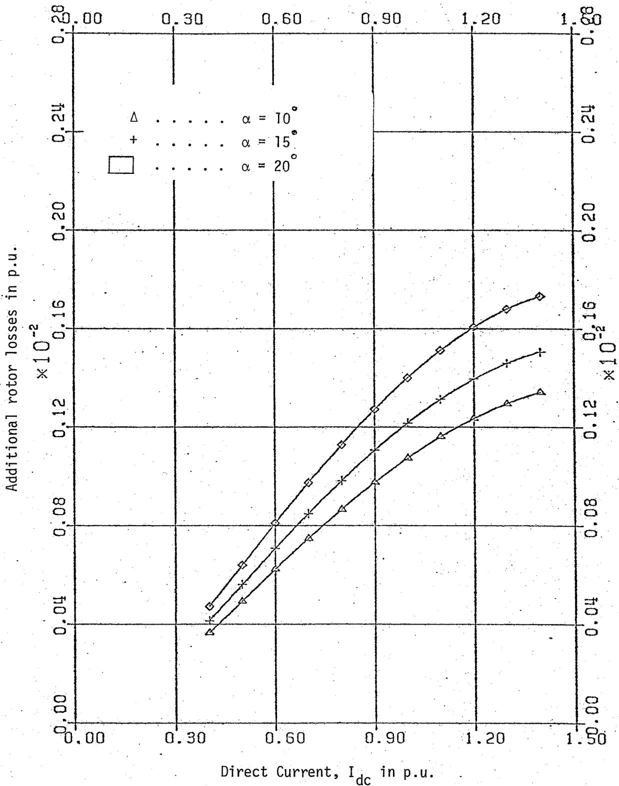
Fig. 3.4 Additional rotor losses of a generator as a function of  $I_{dc}$  in SB connection.
