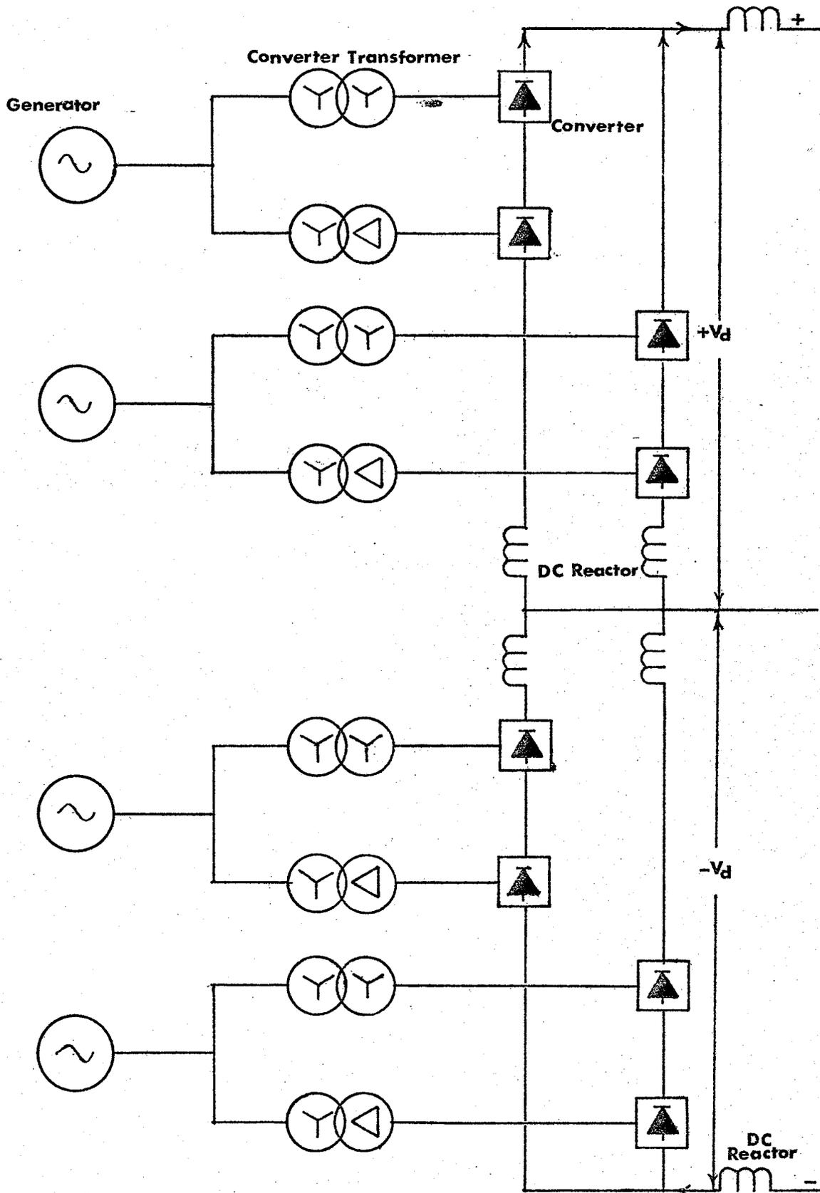
Fig. 5-1 Unit arrangement with parallel connection of bridges
