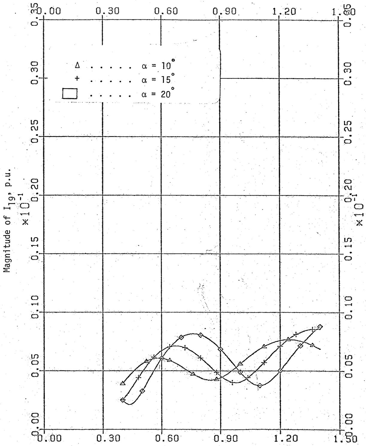
Fig. 2.8 Magnitude of 19th harmonic current as a function of  $I_{dc}$  in SB connection.
