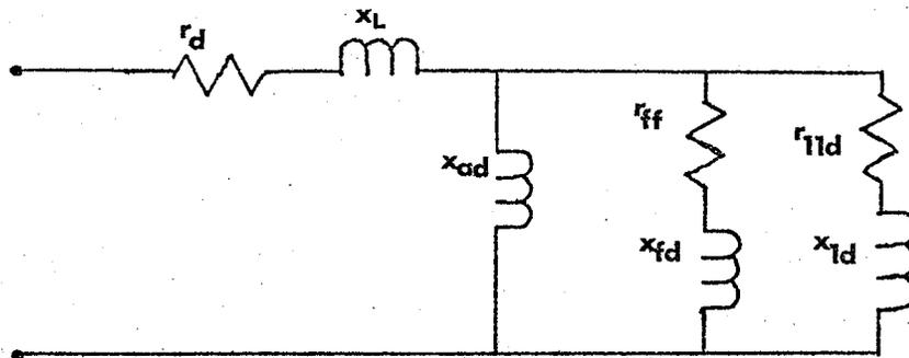
Fig 3-3(b) Equivalent circuit d-axis
