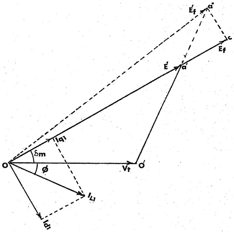
Fig 3.2 (a) Steady state phasor diagram of a synchronous generator
