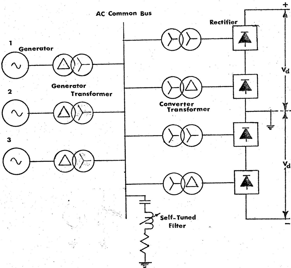
Fig 1.2 Conventional layout of converter stations
