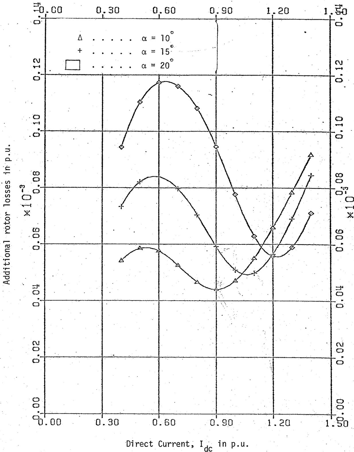
Fig. 3.5 Additional rotor losses of a generator as a function of  $I_{dc}$  in  $\Delta$  connection.
