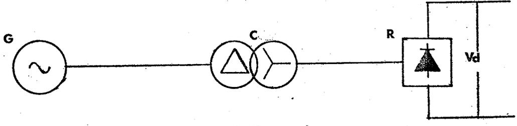
Fig 1-3 (a) Single-Block Connection
