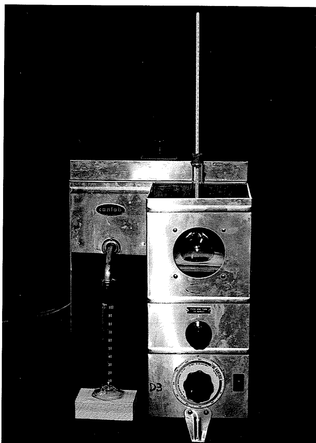
Figure 3.6. An ASTM distillation apparatus for Petroleum fuels.
