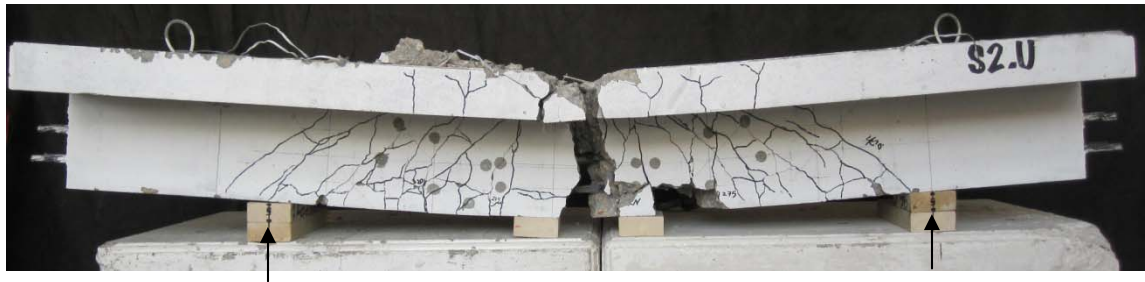
Figure 5- 6: Failure profile of PR-U beams
