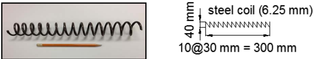
Figure 4- 7: End zone reinforcing coils specifications
