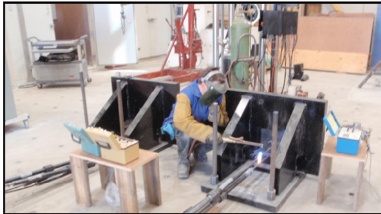
Figure 4- 14: Releasing the prestressing force
