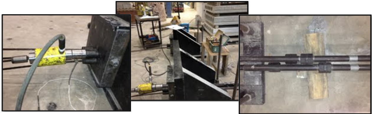
Figure 4- 13: Prestressing setup on the live end
