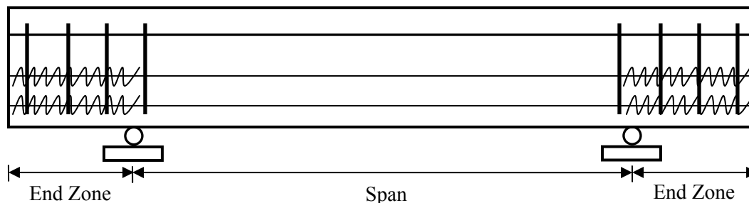
Figure 4- 1: Reinforcement details in the end zones
