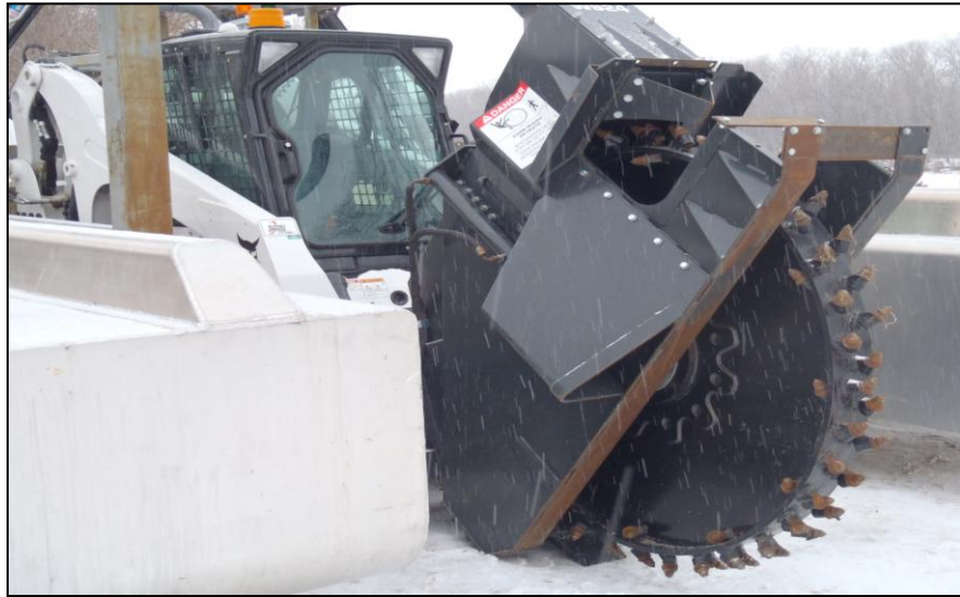
Figure 7.3: The Wolverine used to pre-cut ice covers prior to natural break-up.
