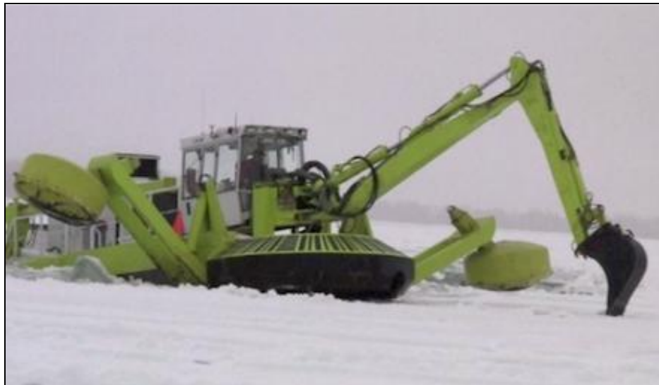
Figure 7.4: Amphibex ice breaker unit.
