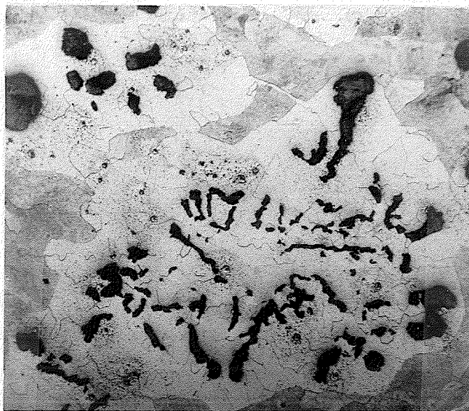
Fig. 17-B Microstructure of as-cast ductile iron casting No. 2 Section B. x 100, 3% Nital etched.
