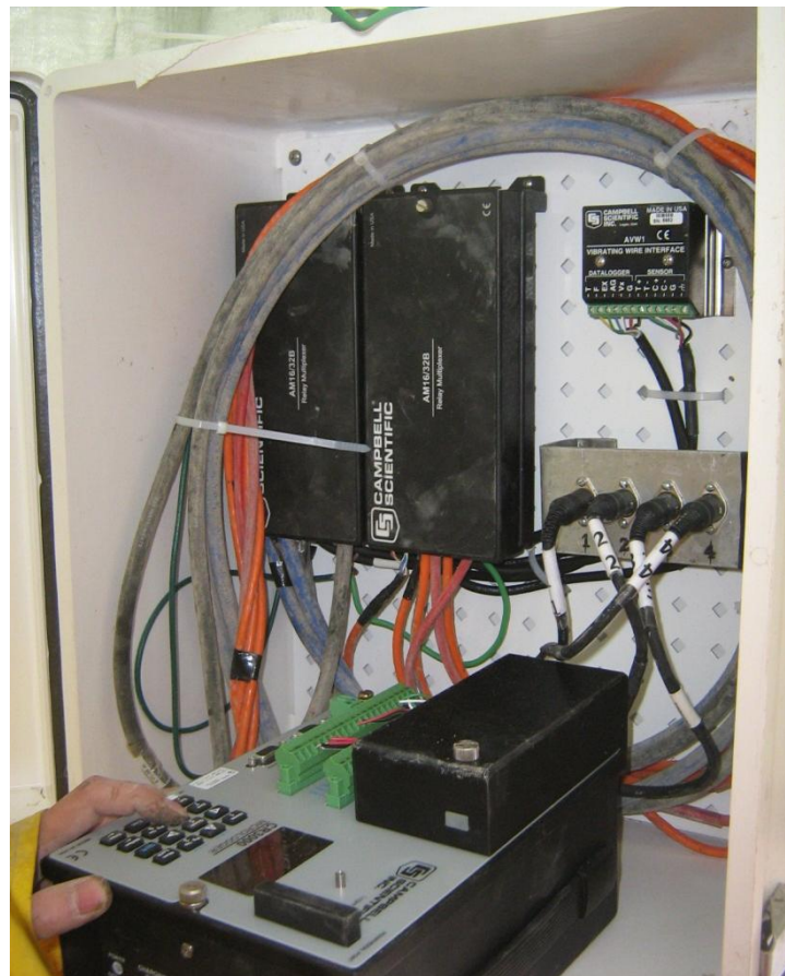
Figure 3.20: Campbell Scientific CR3000 and multiplexers
