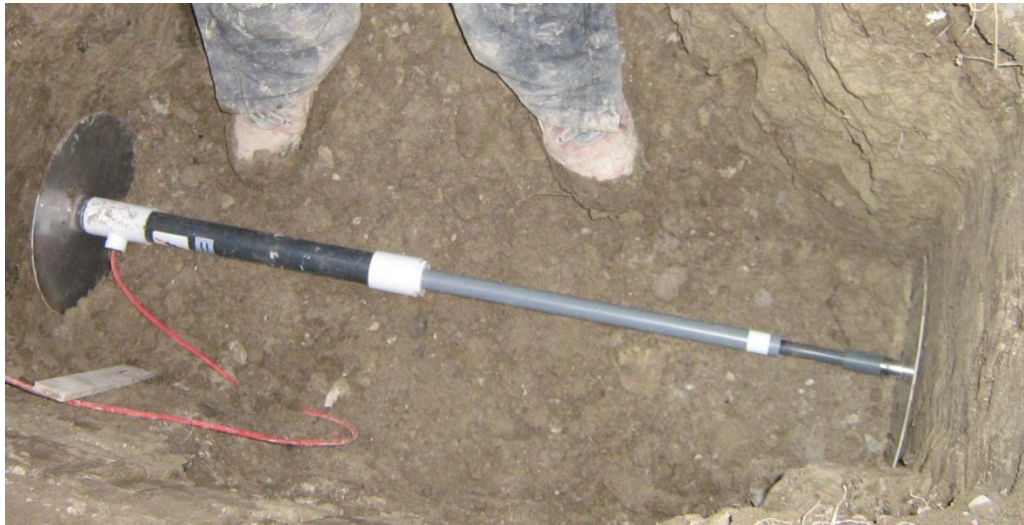
Figure 3.19: Vibrating wire extensometer
