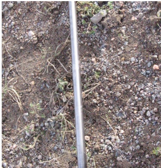
Figure 3.15: Deep settlement gauge
