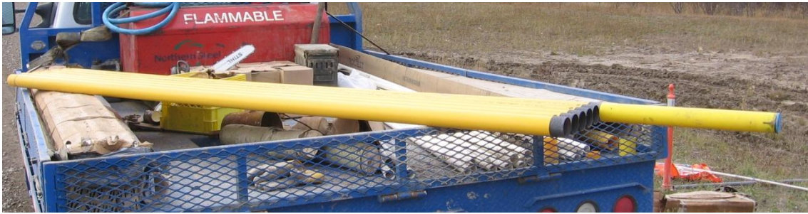
Figure 3.16: Slope inclinometer casings
