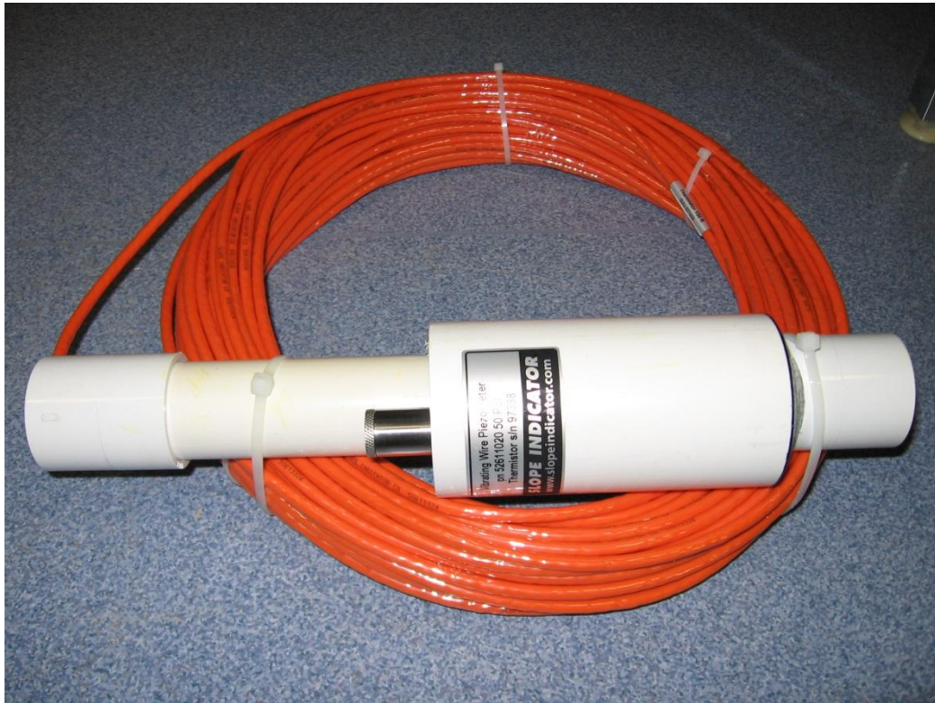
Figure 3.12: Multi-level vibrating wire piezometer
