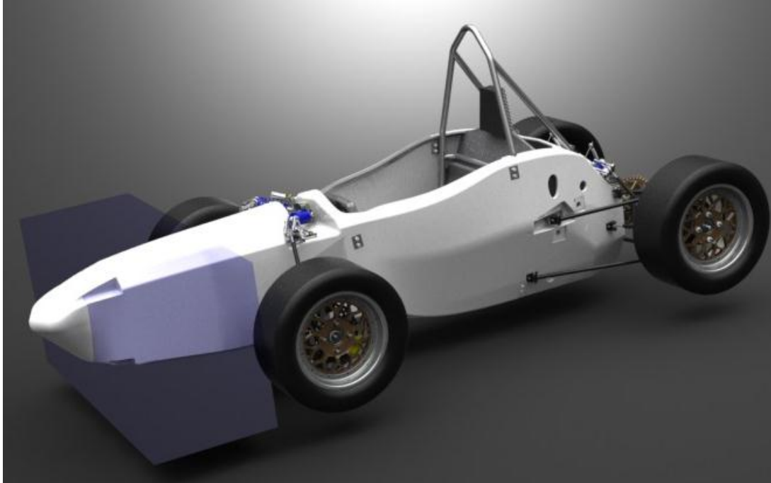
Figure 12. Volumetric Design Boundary resulting from SAE rules and Clearances specified by the UMSAE Electric Team [5].
