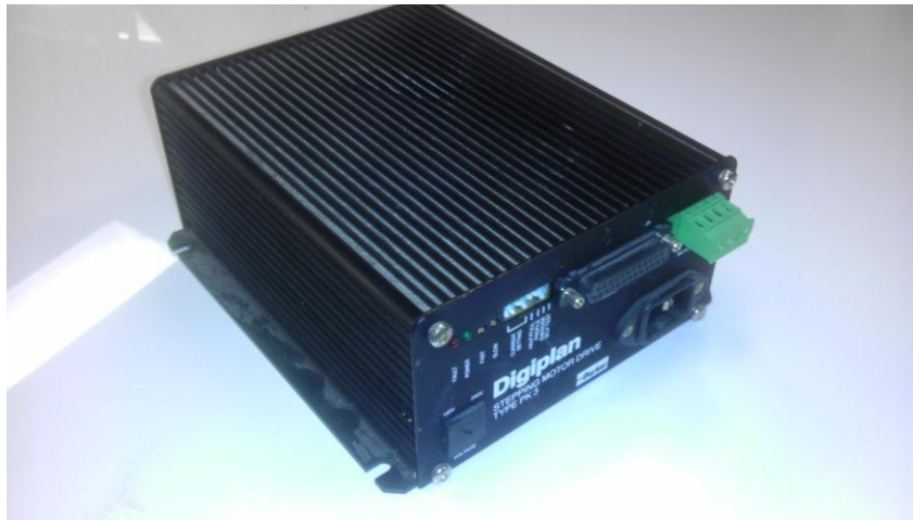
Figure 34. Parker PK3 Stepper Motor Drive – 6.5”x7.0”x3.0” [34].
